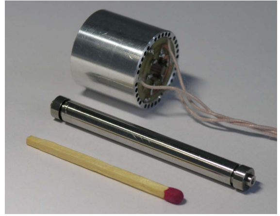
Figure 15. One stator and the common rotor with mounted ball bearings of the test bench.
