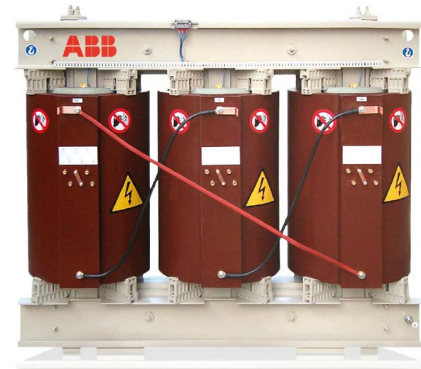
1 MVA – 12kV/400V @ 2600kg 0.2%/1% Losses @ No/Rated Load
