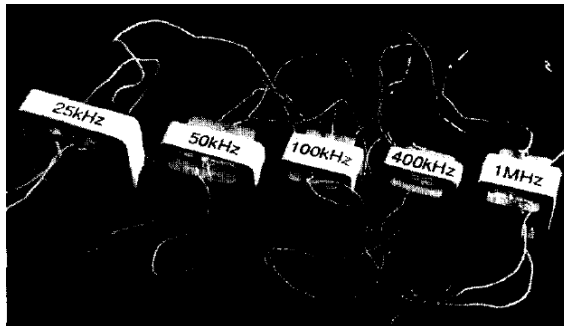
Transformer Volume &amp; Weight vs. Frequency
