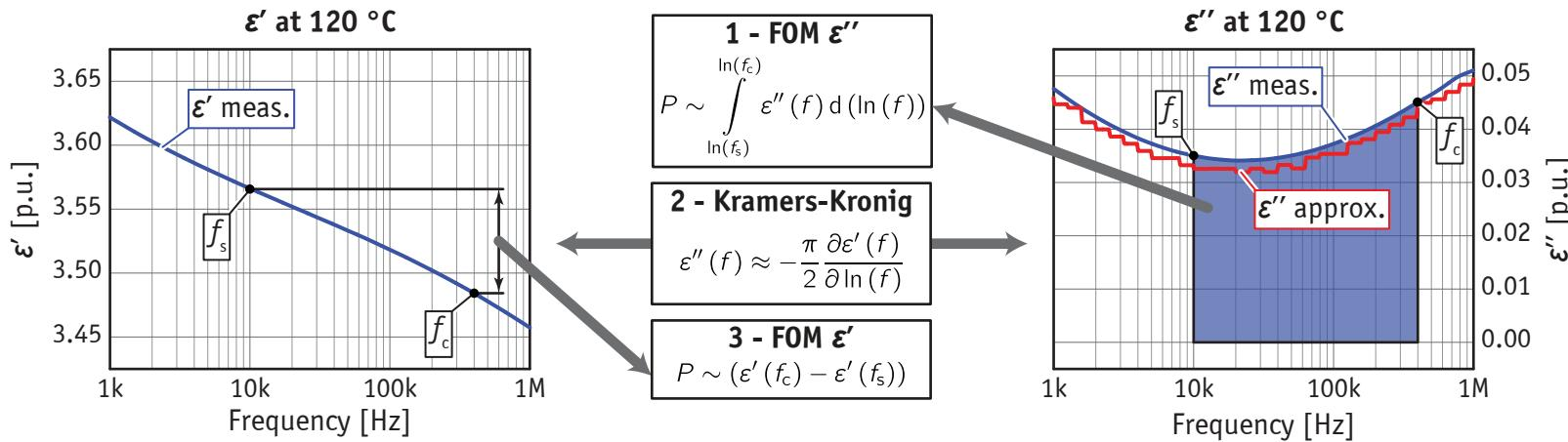
$$f_s = 10.0 \text{ kHz} / t_r = 800 \text{ ns} / D_c = 0.5 / T = 120 \text{ °C} / \text{Damsol 3418}$$
