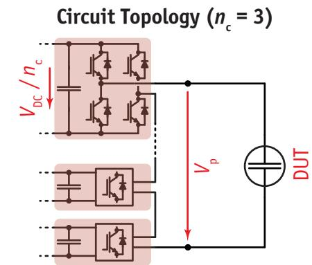
$$f_g = 50 \text{ Hz} / f_s = 10.0 \text{ kHz} / t_r = 100 \text{ ns} / P' = P / (\epsilon'' \cdot C_0 \cdot V_{DC}^2) = P'_1 + P'_{\text{harm}}$$
