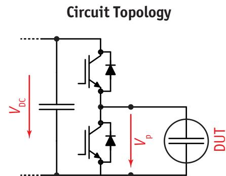
$$f_s = 10.0 \text{ kHz} / t_r = 100 \text{ ns} / D_c = 0.5 / P' = P / (\epsilon'' \cdot C_0 \cdot V_{DC}^2)$$
