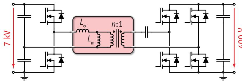
▼ 400 V SiC Test Converter
