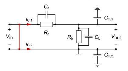
$C_{C,1}$  causes CM current in  $C_b$  and  $C_a$
