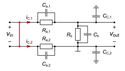
Non-symmetrical  $C_{C,1}$  and  $C_{C,2}$  cause a common mode current in  $C_{b}$
