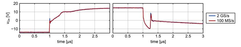
Zoom view: the sampling rate of 100 MS/s affects the measured signal observably; at 200 MS/s, the impact of the sampling rate gets negligible
