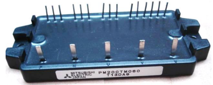
Mitsubishi Electric IGBT module with integrated current sense IGBT and corresponding terminals
