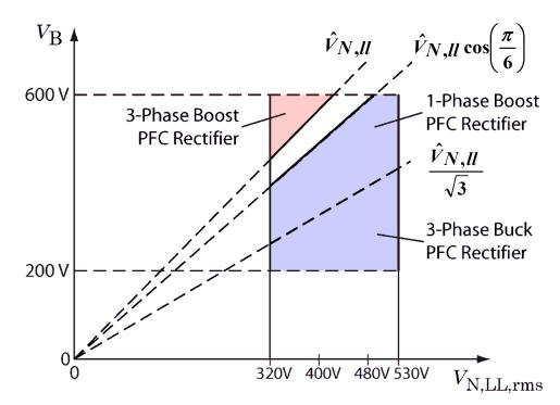
$V_{\rm B}$  ...... Battery Voltage  $V_{\rm N,ll,rms}$  ... RMS Value of Mains Line-to-Line Voltage
