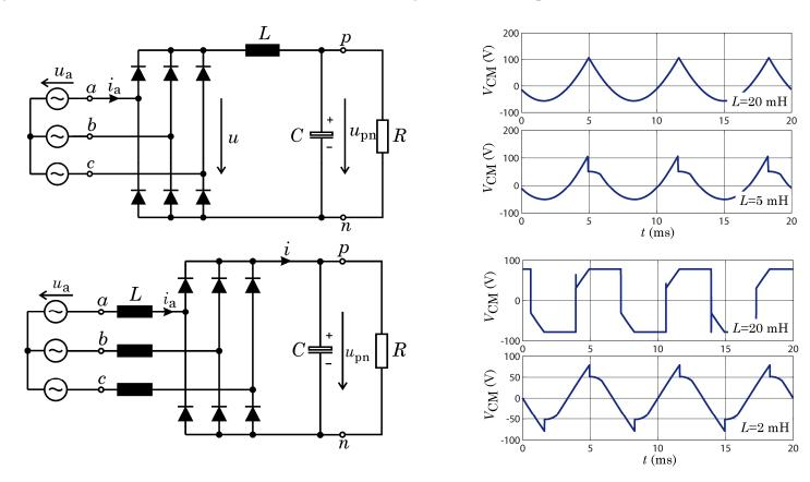
Output shows Low-Frequency Common Mode Voltage; Load / Battery cannot be Connected to Ground (Isolation Required)
