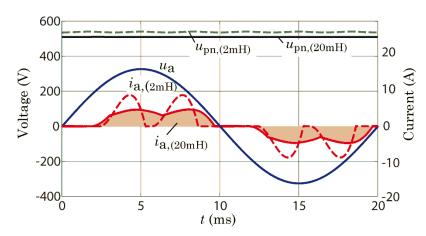
$U_{LL} = 3 \times 400 \text{ V}$   $f_{N} = 50 \text{ Hz}$   $P_{O} = 2.5 \text{ kW (R=125 }\Omega)$  C = 1 mFL = 2 mH; 20 mH
