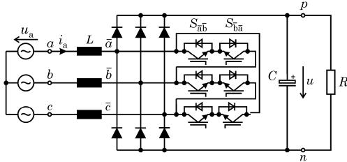
AC Side Equivalent Circuit
