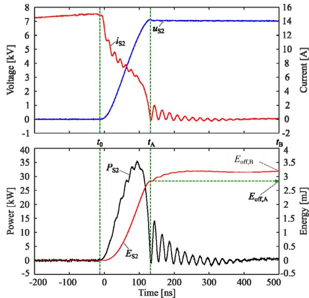
► Accurate Calorimetric Method for Ultra-Fast Semiconductors
