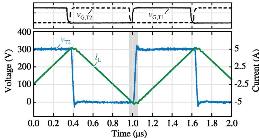
► **90% Switching Loss Reduction** compared to Hard-Switching
