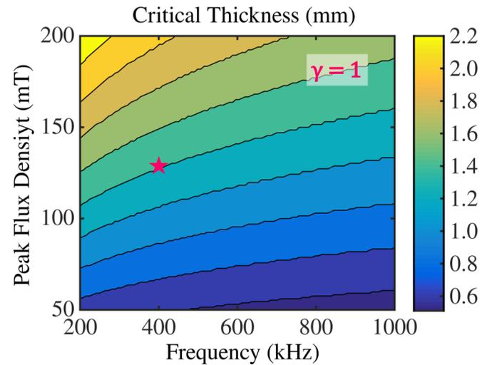
▲ 3F4 Critical Thickness For Obtained SE Parameter at 125 mT / 400 kHz
