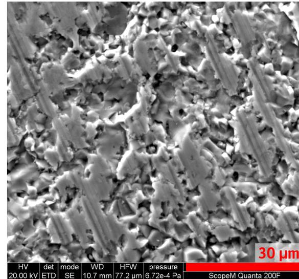
▲ SEM Image of Surface Condition of MnZn Ferrite (3F4) After Machining
