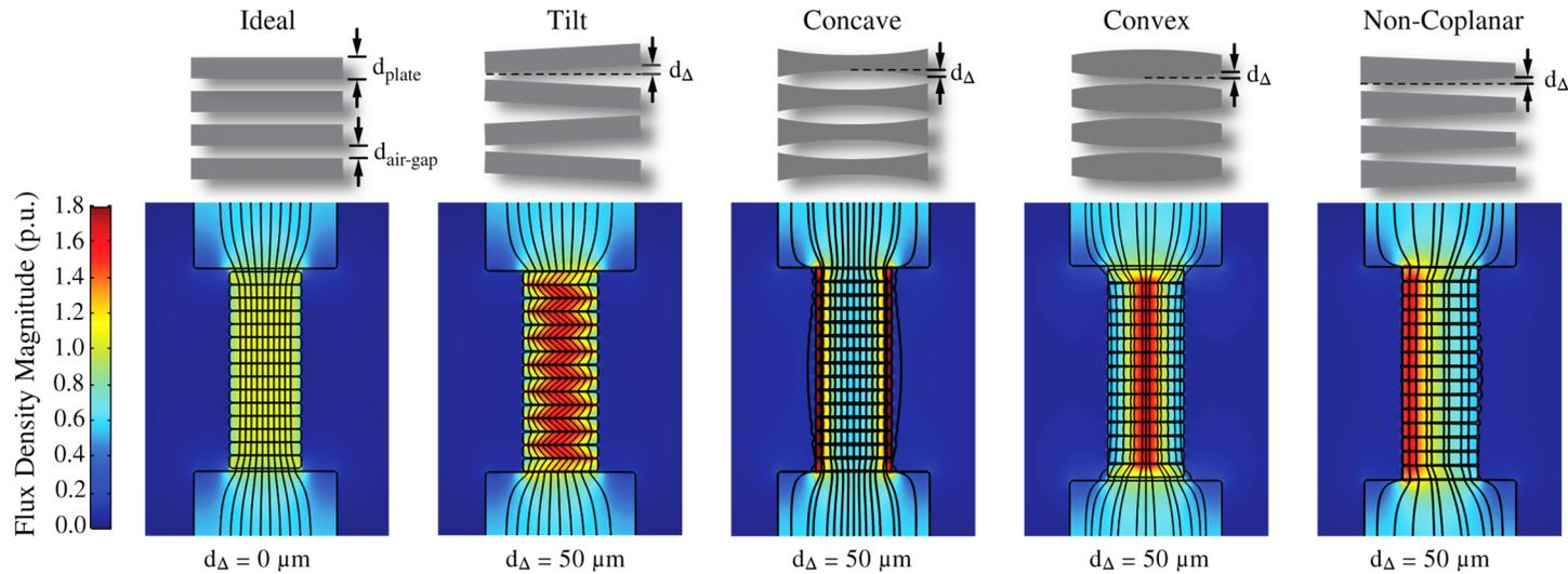
▲ 2D FEM Showing Non-Homogeneous Flux Density Distribution Caused By Mech. Tolerances
