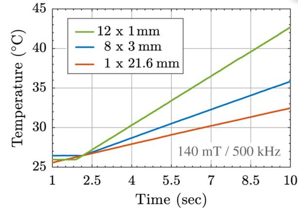
▲ Temperature Rise For Plates W/ Different Thickness
