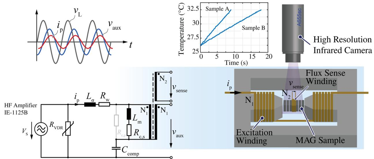
▲ Temp. Rise Monitoring of Ferrite Sample W/ Infrared Camera
