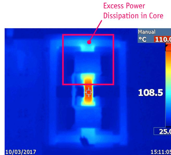
▲ Temp. Rise Of Prelim. Test Circuit With 20 AG Sample. 100mT/500 kHz For 90 Sec.
