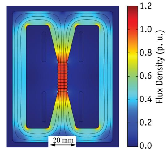
▲ FEM Simulation of Flux Density Distribution in Test Circuit And Sample
