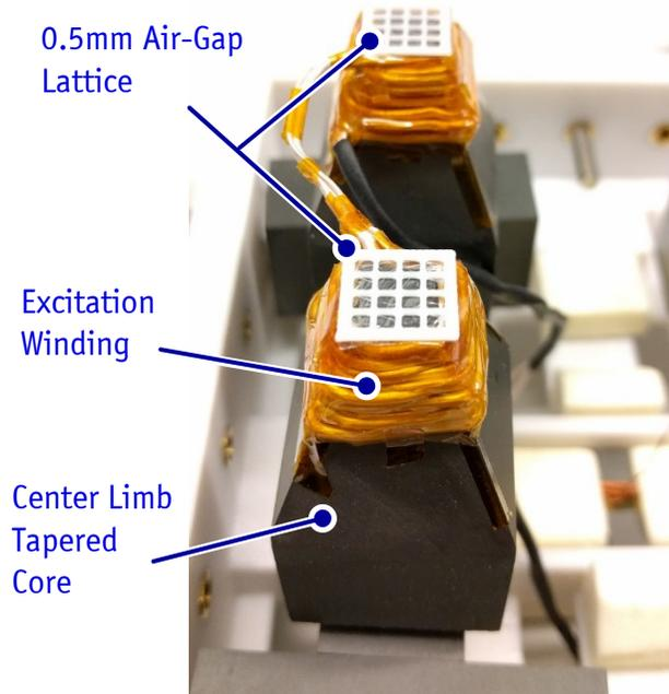
▲ Tapered Center Limb Core With Air-Gap Lattice
