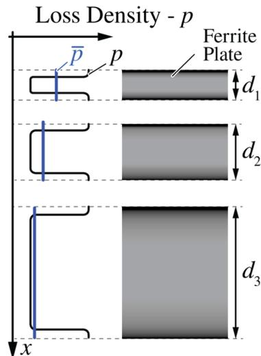
▲ Avg. Loss Density Depends On Plate Thickness
