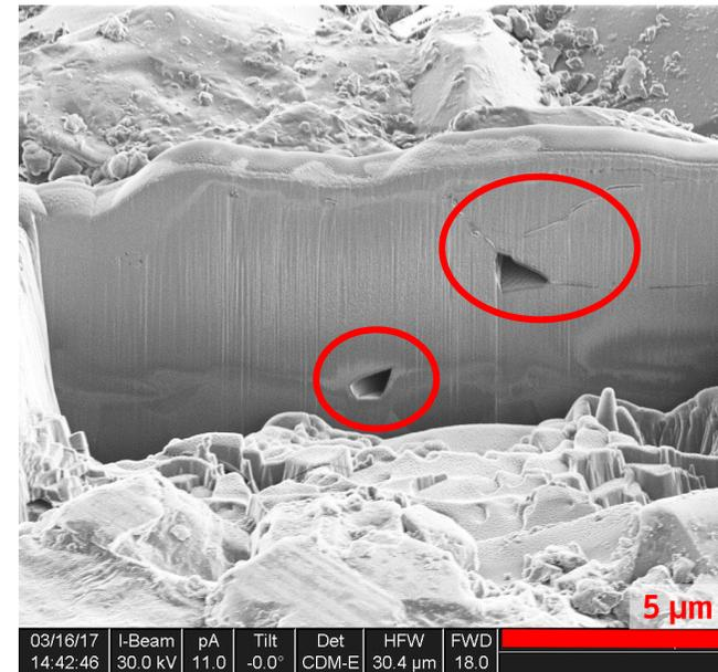
▲ FIB-SEM Images Revealing Subsurface Condition of Machined MnZn Ferrite (3F4)
