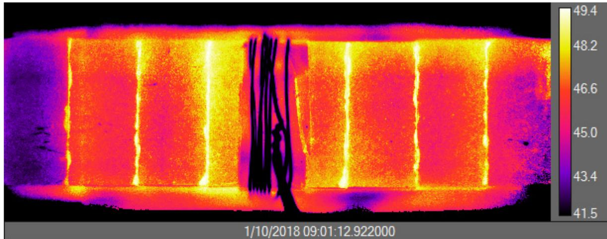
▲ 3F4 MAG Sample (8 x 3mm) Temperature Rise Snapshot at 47 °C Avg. Sample Temperature
