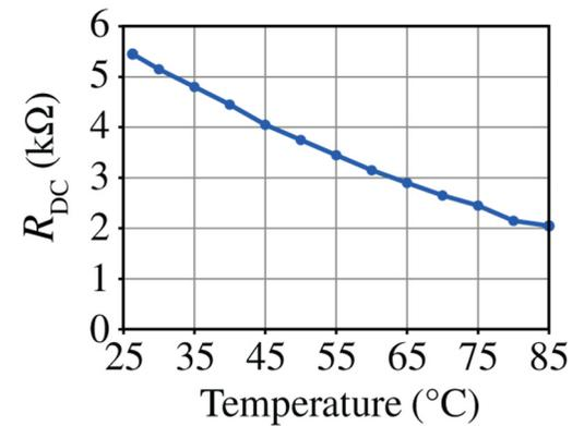
▲ DC Resistance of 3F4 MnZn Ferrite as a Function of Temperature
