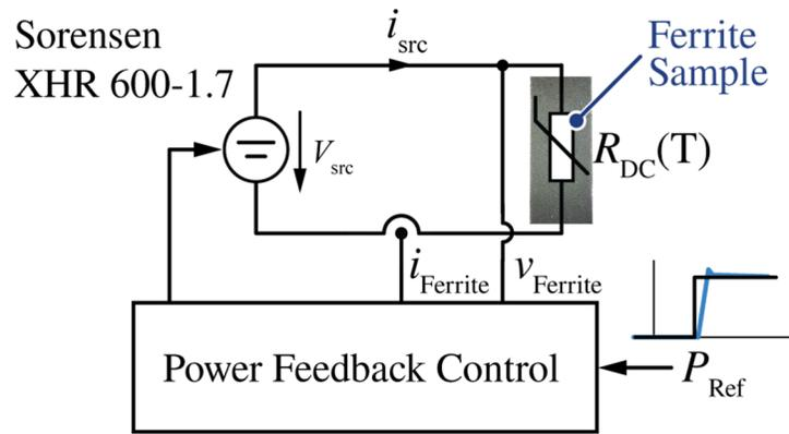
▲ Feedback Control of DC Power Dissipation in Ferrite
