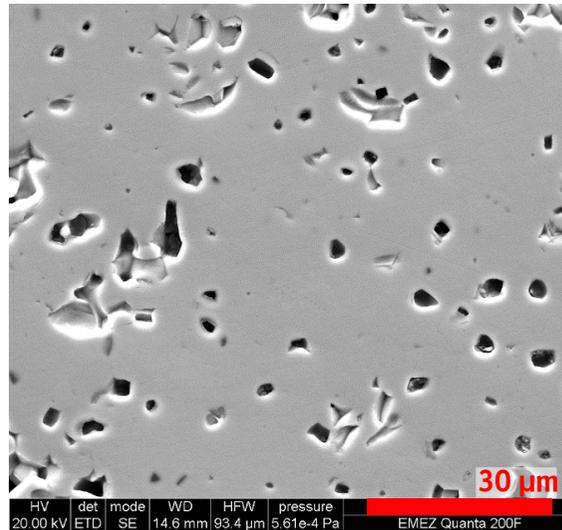
▲ SEM Images of MnZn Ferrite (3F4) After Removing 500 μm Thick Layer at Surface
