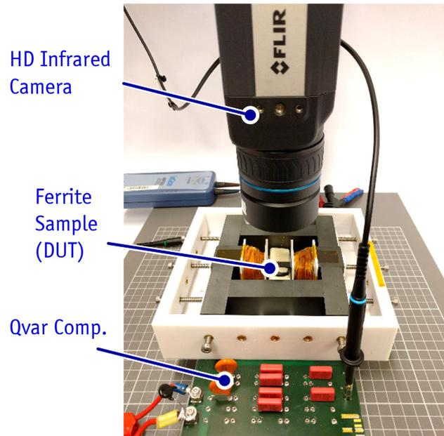
▲ Surface Loss Test Setup W/ Res. Cap. Bank and Infrared Camera
