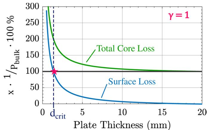
▲ 3F4 Critical Thickness For Obtained SE Parameter at 125 mT / 400 kHz
