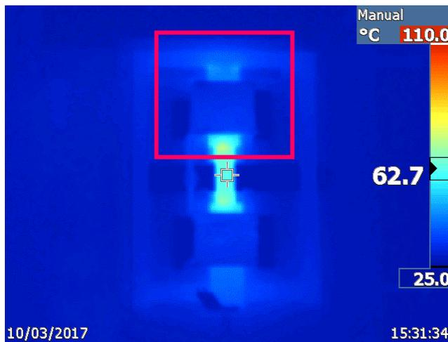
▲ Temp. Rise Of Prelim. Test Circuit With Solid Sample. 100mT/500 kHz For 90 Sec.
