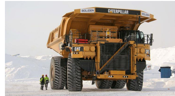
Caterpillar 797F — 350 tons payload / 3 MW
