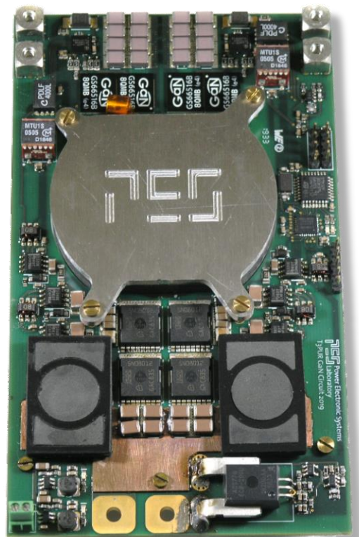
Fig. 3: Three-port resonant converter employing the CFFC concept.
