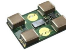
Source: R. Pilawa Integrated Dual-Sided Half-Bridge Flying Capacitor Converter Switching Cell
