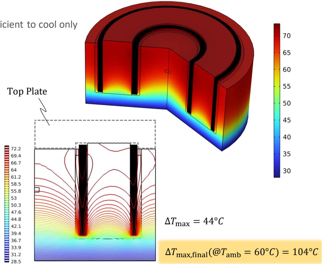
► **Simplified Heat Sink Design** using an aluminum plate only
