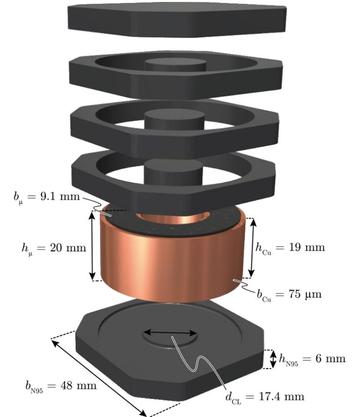
► **Transformer Dimensions** and winding arrangement of the foil winding transformer
