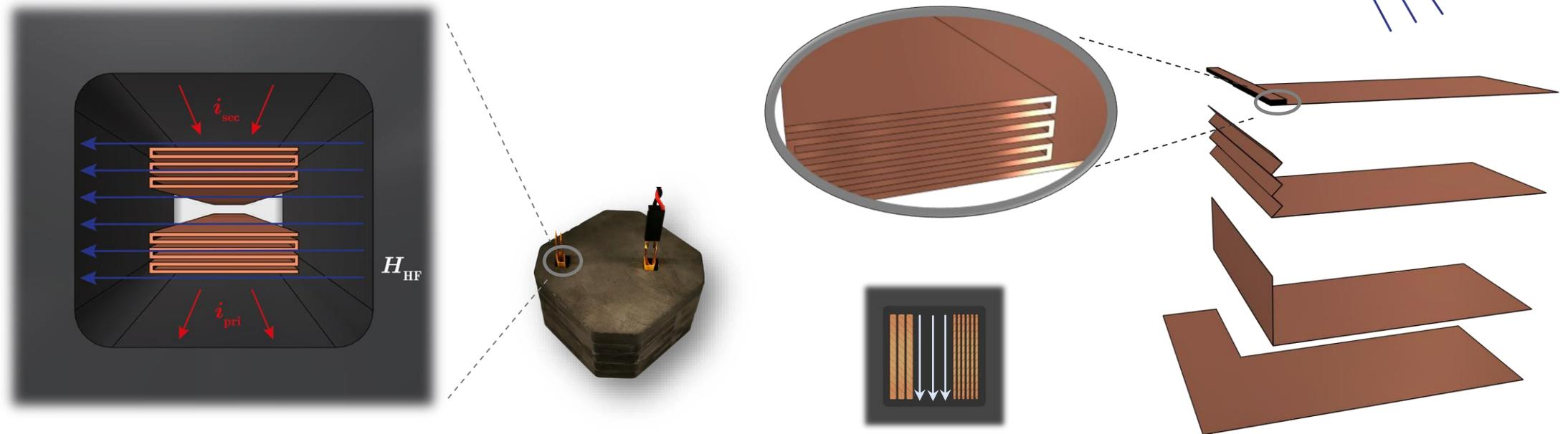
► **Magnetic Field Distribution** in the cutouts in the transformer core for the winding terminals
