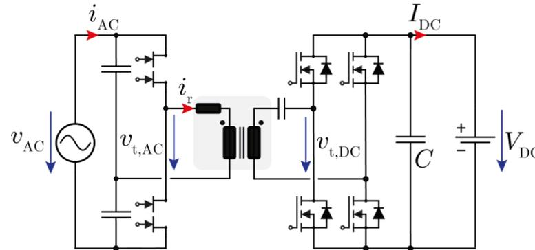
► Bidirectional Isolated AC/DC Converter (Buck/Boost)
