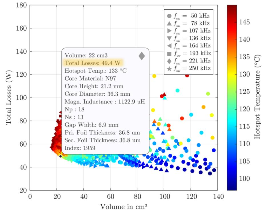
► Optimization Results of the foil winding transformer with M3+ Kapton tape, where thermally unfeasible designs are discarded
