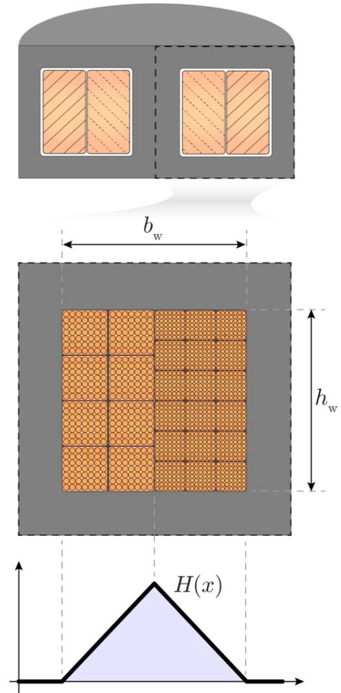
► **Conduction Losses per Leakage Inductance** in a pot core transformer with litz wire (40um) windings for different geometrical parameters
