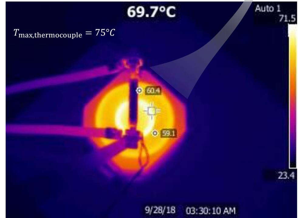
► **Simplified Heat Sink Design** using an aluminum plate only
