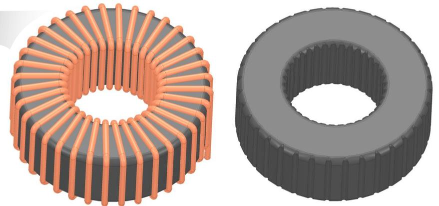
► **FEM Simulation Result** of a toroidal inductor arrangement suitable for the measurement of the relative permeability and the core losses of a material
