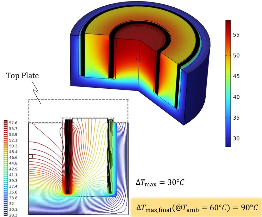
► **Heat Sink Design** of achieving minimal hot spot temperatures
