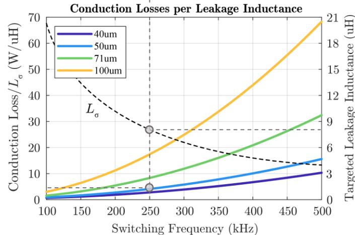
► **Conduction Losses per Leakage Inductance** for different strand diameters, switching frequencies and an RMS current of 18 A
