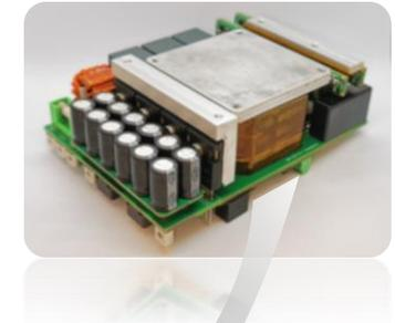
⇒ Due to the model's **overestimation** of the **hotspot temperature**, it is sufficient to cool only **one side** of the transformer
