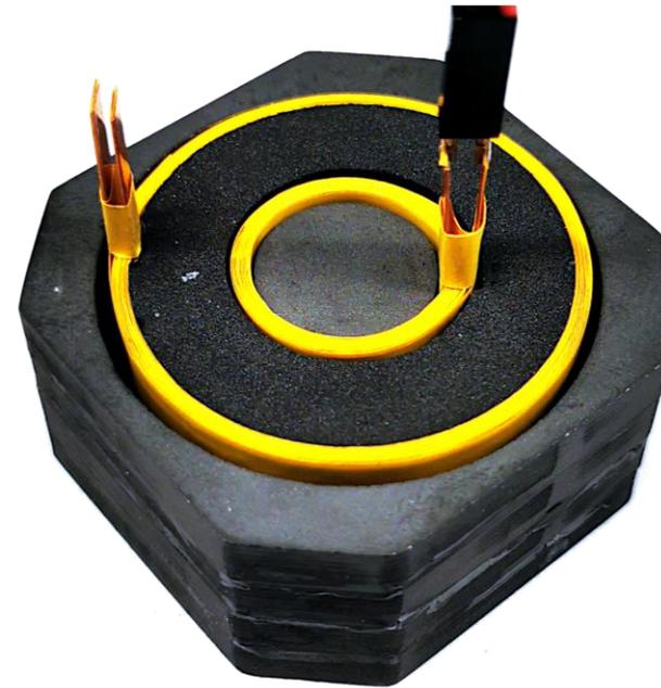
► **Completely Assembled Transformer** without top plate and potting of the winding
