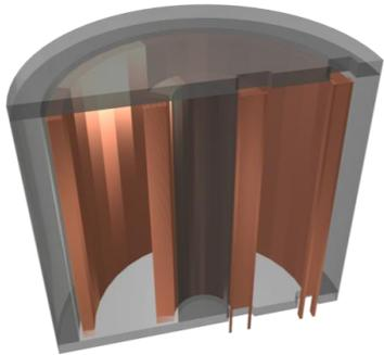
$$L_{\sigma, \text{foil}} = \frac{\mu_0 N_p^2}{3h_w} \cdot (l_{w,p} d_{w,p} + 3l_{w,\text{gap}} d_{w,\text{gap}} + l_{w,s} d_{w,s})$$
