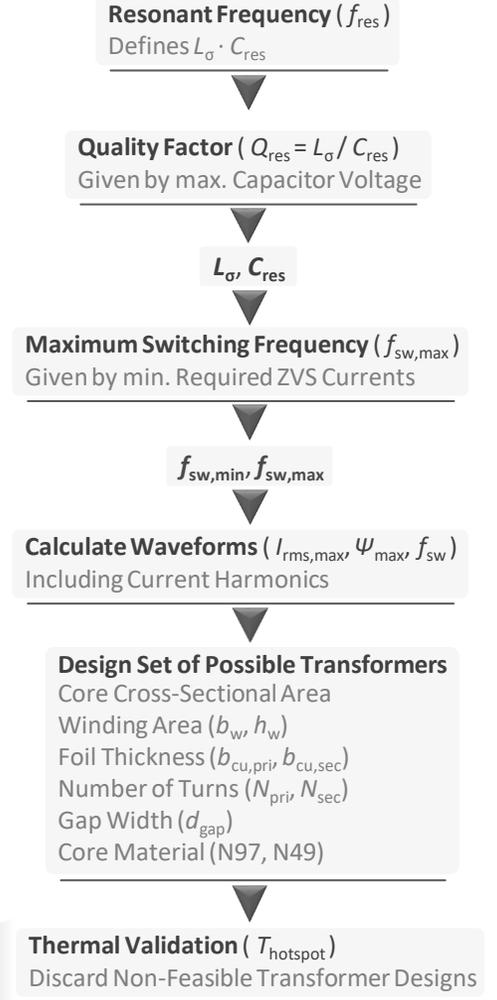
► **Thermal Model** for estimating the temperatures in foil winding transformers for certain given conduction and core losses
