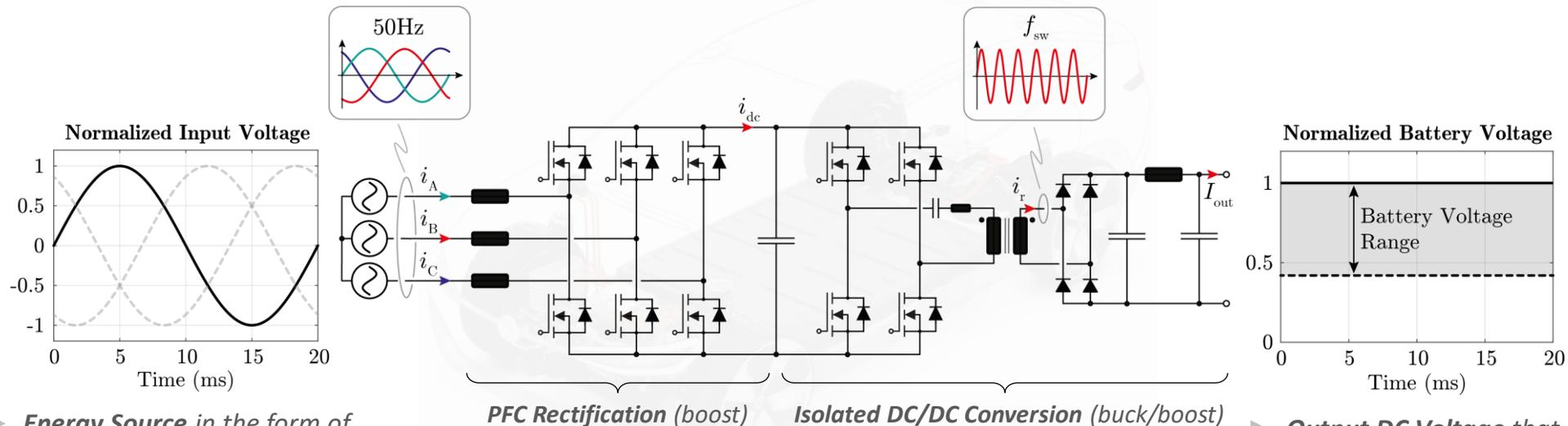
► **Energy Source** in the form of a single-phase or three-phase AC voltage grid
