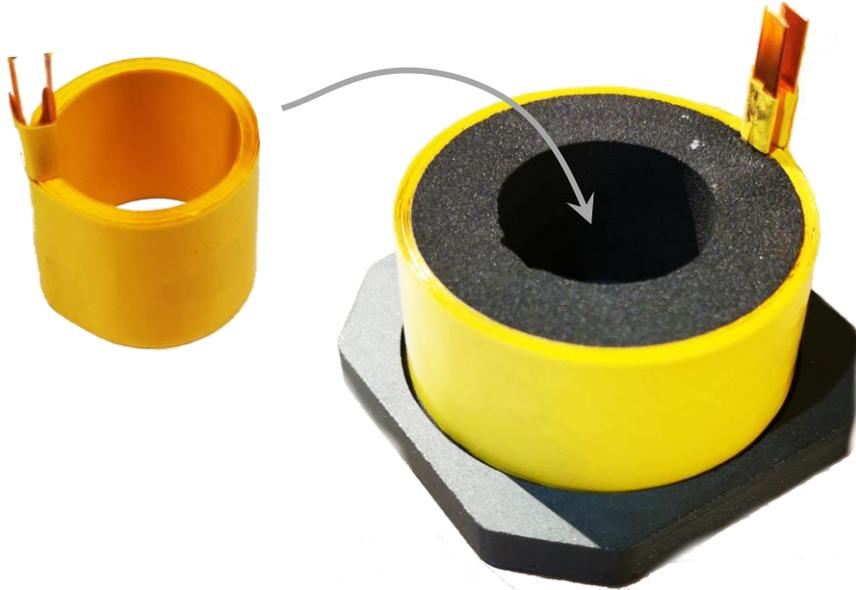
► **Winding Assembly** of the two foil windings with the low permeability ring in between
