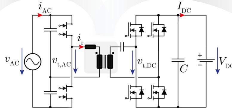
► Bidirectional Isolated AC/DC Converter (Buck/Boost)
