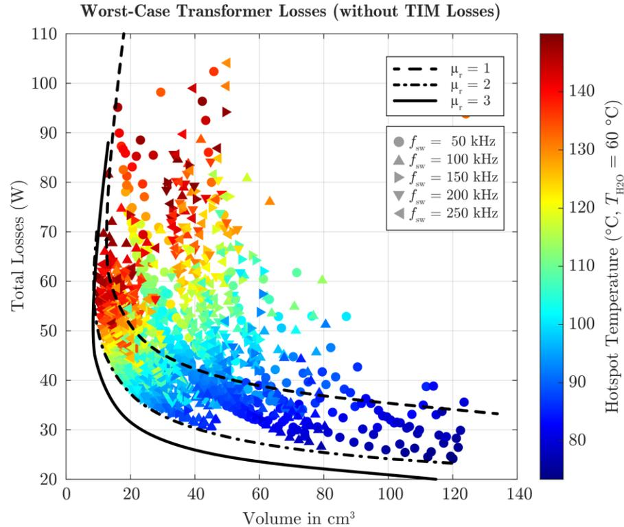
► Optimization Results of the foil winding transformer with M3+ Kapton tape, where thermally unfeasible designs are discarded
