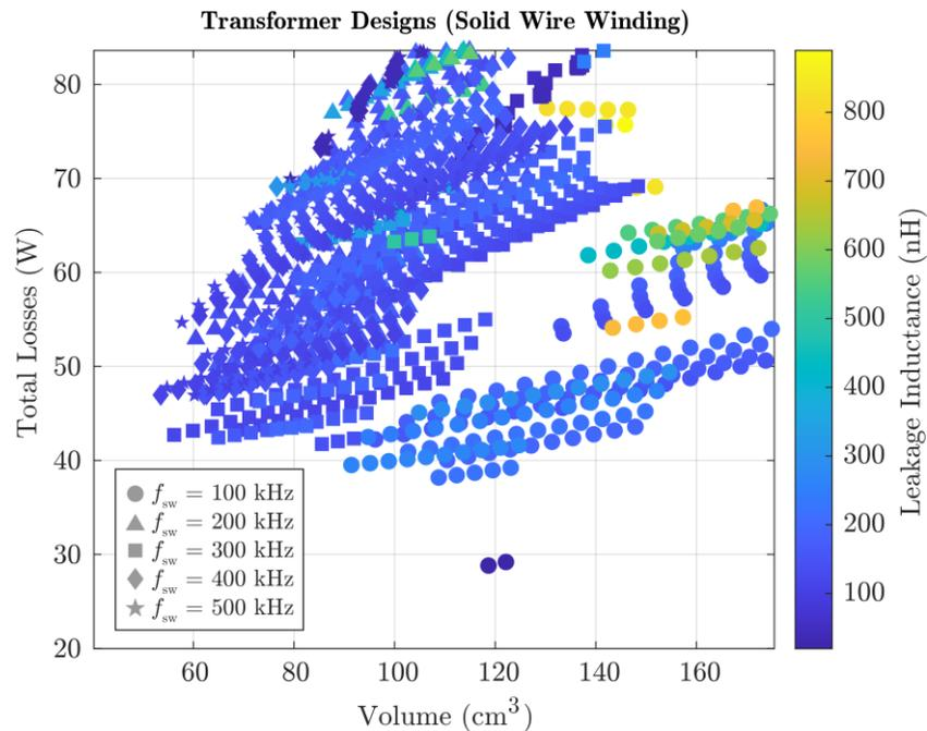
► **Maximum Leakage Inductance** in solid wire winding transformers for different switching frequencies
