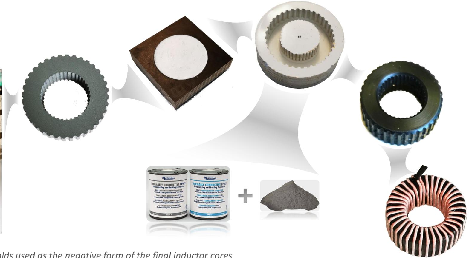
► *Manufacturing Sequence of the silicone molds used as the negative form of the final inductor cores*
