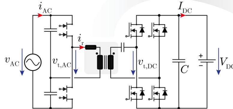
► Bidirectional Isolated AC/DC Converter (Buck/Boost)
