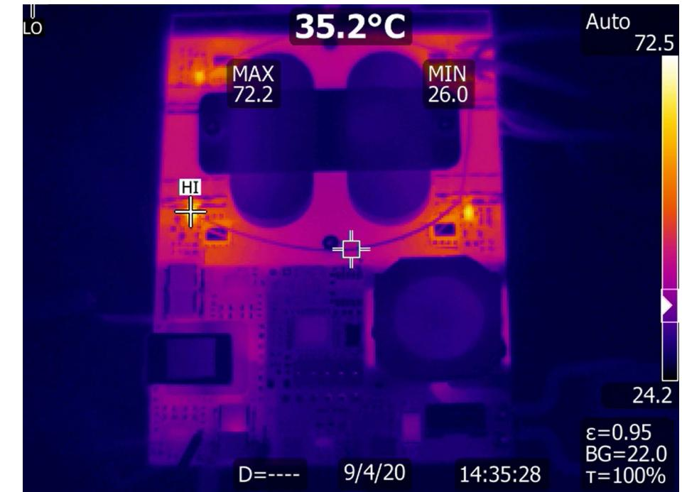
■  $V_{dc} = 400 \text{ V}$ ,  $V_o = 12 \text{ V}$ ,  $P_o = 1.5 \text{ kW}$
