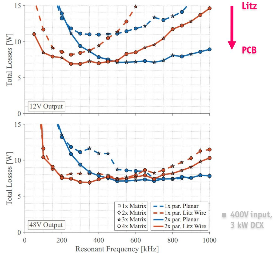
Source: M. Kasper et. al., "Ultra-high Power Density Server Supplies Employing GaN Power Semiconductors and PCB-Integrated Magnetics", Proc. CIPS 2020
