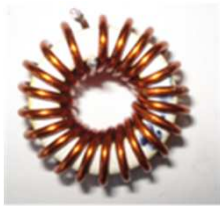
DM Inductor: Micrometals T94-26 Iron Powder Core, 21 turns, \phi_w=1.5\text{mm}
