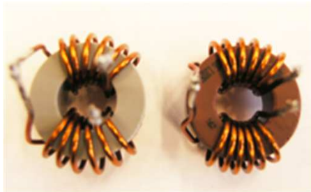
CM Inductor: Air/ VAC Vitroperm 500F Nanocrystalline Core, 2x7 turns, \phi_w=1.5\text{mm}
