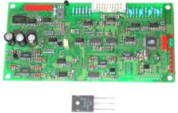
Fig.6: Control board of the VIENNA Rectifier in comparison with a TO247-type power semiconductor package. The overall dimensions of the control board are 16\text{cm} \times 8\text{cm} ( 6.3\text{in} \times 3.15\text{in} ).
