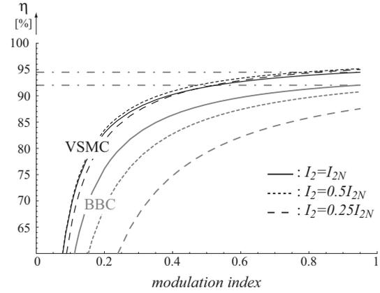
Fig.13 Efficiency comparison of the VSMC and BBCs for unity output power factor and varying output current.
