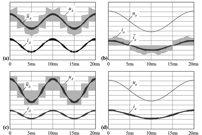
Fig.5 Comparison of the VSMC (a) output and (b) input waveforms and the BBC (c) output and (d) input waveforms operating at the nominal output power of 6.8kW. Output voltages shown include the instantaneous output voltage and averaged output voltage. Scales: 150V/div, 15A/div.
