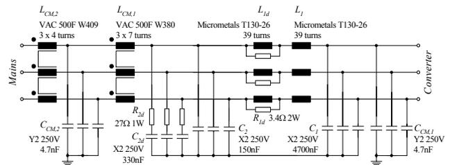
Fig.10 EMC input filter schematic for the BBC system and is designed to comply with CISPR 11 class B requirements.
