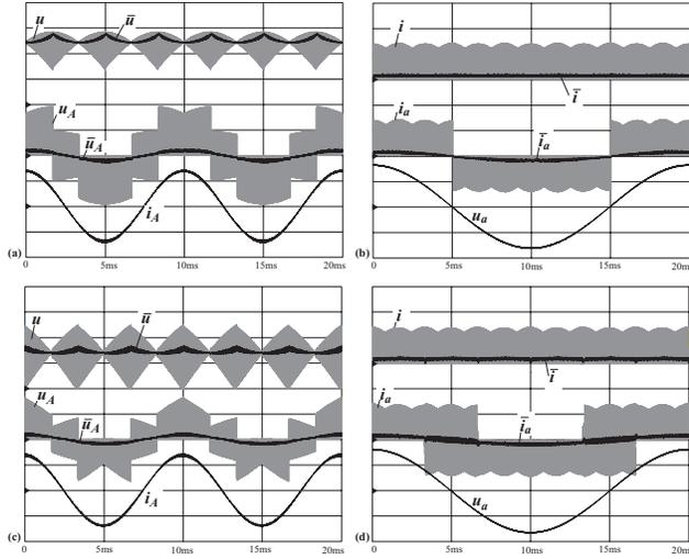
Fig.3 Simulation of the VSMC operating behavior for *MS1* (a)&(b) and *MS2* (c)&(d); (a)&(c) DC link voltage  $u$ , local average  $\bar{u}$ , output phase voltage  $u_A$  (w.r.t load star point), local average  $\bar{u}_A$ , output phase current  $i_A$ ; (b)&(d) DC-link current  $i$ , local average  $\bar{i}$ , input phase current  $i_a$ , local average  $\bar{i}_a$ , input phase voltage  $u_a$ ; scales: 200V/div, 15A/div;  $M_{12}=0.1$ ,  $\Phi_2=0$ .
