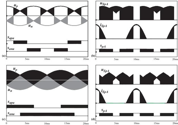
Fig.4 Modulation of the VSMC input and output stage for *MS1* (a)&(b) and *MS2* (c)&(d) for output current phase displacement  $\Phi_2=0$ . Representation of positive and negative DC link bus,  $u_p$  and  $u_n$ , w.r.t the mains star point ((a)&(c)) and switching functions  $s_{apa}$  and  $s_{ana}$  of input stage bridge leg  $a$ ; also shown: voltage, current and switching function of transistor  $S_{pA}$  on VSMC output stage.
