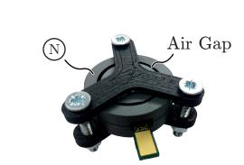
▶ PCB inductor using new design approach (L = 5uH)
