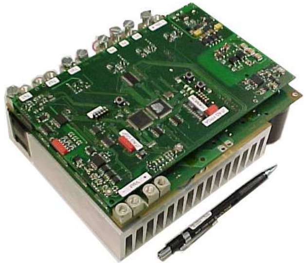
Figure 15: Converter with the inverter, the fourth leg and the active rectifier.
