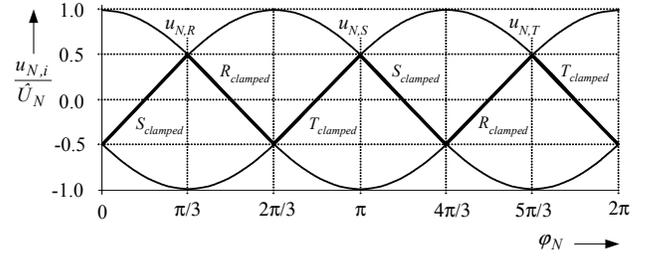
**Fig.3:** Time behavior of the mains phase voltages  $u_{N,i}$ ,  $i=R,S,T$ ; the power transistor of the phase showing the lowest absolute instantaneous voltage value, e.g.  $S_S$  in  $0 < \varphi_N < \pi/3$ , is clamped in the on-state.
