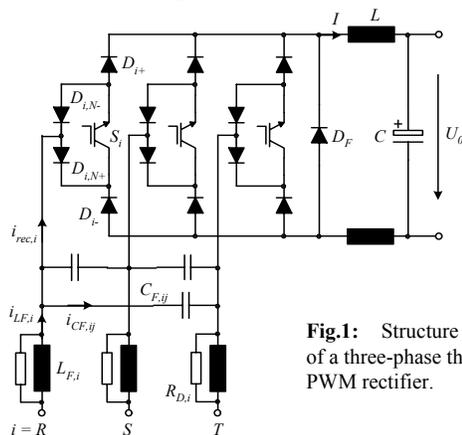
**Fig.1:** Structure of the power circuit of a three-phase three-switch buck-type PWM rectifier.
