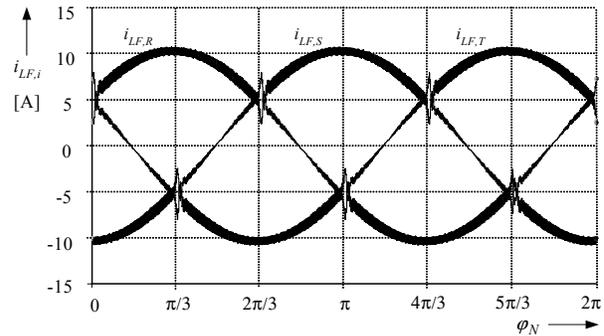
**Fig.2:** Distortion of the mains phase currents of a three-phase three-switch buck-type PWM rectifier occurring for conventional PWM at the limits  $\varphi_N = n\pi/3$  ( $n = 1, 2, 3, \dots$ ) of bridge leg clamping intervals (cf. Fig. 3).
