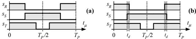
**Fig. 7:** Switching functions of the proposed advanced modulation scheme preventing sliding intersections of the filter capacitor voltages; assumed relations of the mains voltages according to  $0 < \varphi_N < \pi/3$  (cf. also Fig. 4(a)). **(a)** ideal switching state sequence; **(b)** modified switching state sequence considering an overlapping time  $t_d$  when switching over from  $j = (101)$  to  $j = (011)$ .
