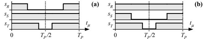
**Fig. 4:** Switching state sequences for one pulse period depicted for two different mains phase voltage conditions: **(a)**  $u_{N,R} > u_{N,S} > u_{N,T}$  and/or  $0 < \varphi_N < \pi/3$  (sector 1), and **(b)**  $u_{N,S} > u_{N,R} > u_{N,T}$  and/or  $\pi/3 < \varphi_N < 2\pi/3$  (sector 2).
