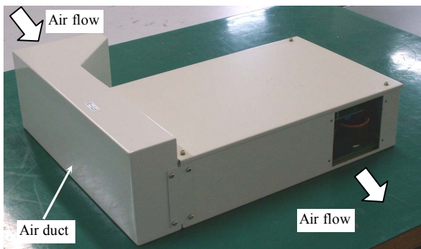
Fig.9. The external appearance of 1kw grid-connected converter
