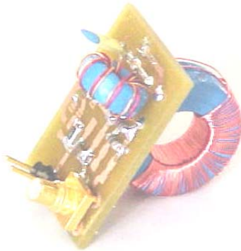
Fig.11: Prototype of the proposed current sensor.
