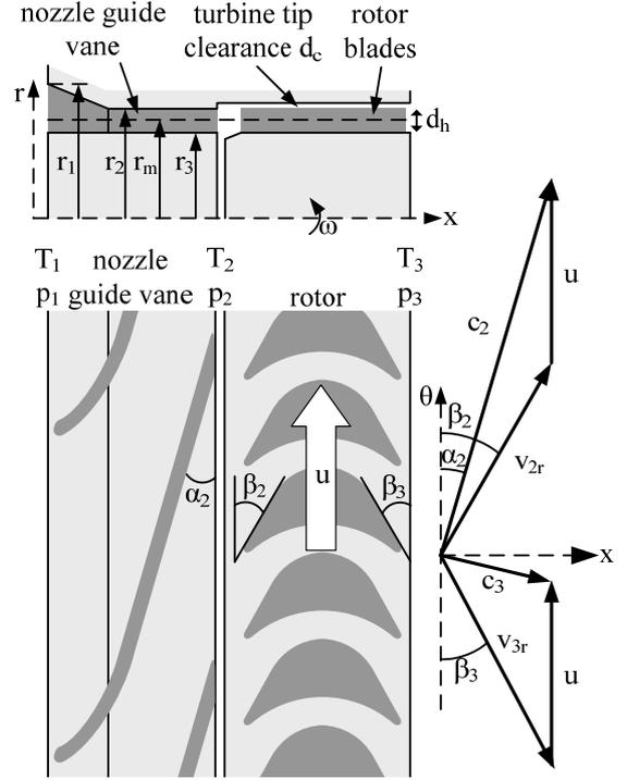
Fig. 2. Drawing of the single-stage axial impulse turbine (Laval turbine) with  $r_m = 4.5$  mm and the corresponding nozzle guide vane and velocity diagrams at rotor inlet and outlet for the rated rotational speed.  $c_2$  and  $c_3$  are the absolute velocities at the rotor inlet and outlet.  $v_{2r}$  and  $v_{3r}$  are the relative velocities at the rotor inlet and outlet.  $u$  is the rotor speed at radius  $r_m$ .
