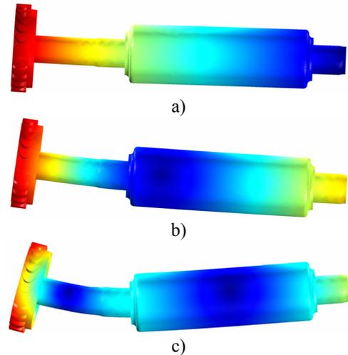
Fig. 5. Bending modes of the rotor. First bending mode at 198 840 rpm, 3314 Hz (a), second bending mode at 285 420 rpm, 4757 Hz (b) and third bending mode at 723 900 rpm, 12065 Hz (c).
