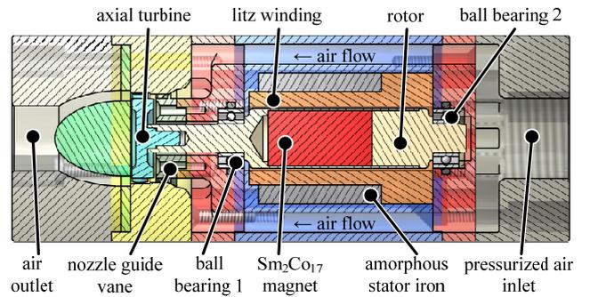
Fig. 4. Solid model of the ultra compact (22 mm x 60 mm) air-to-power demonstrator.
