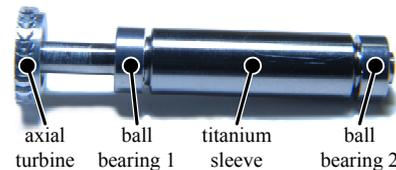
Fig. 6. Impulse turbine and rotor with assembled high speed bearings.
