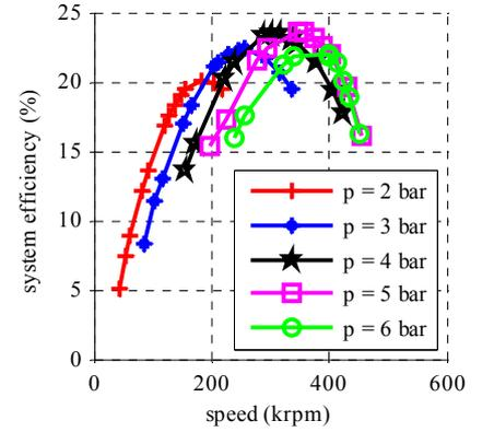
Fig. 12. System efficiency as a function of speed and inlet pressure.
