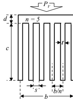
**Fig.1:** Geometry of an extruded heat sink with six fins and five channels ( $n=5$ ).
