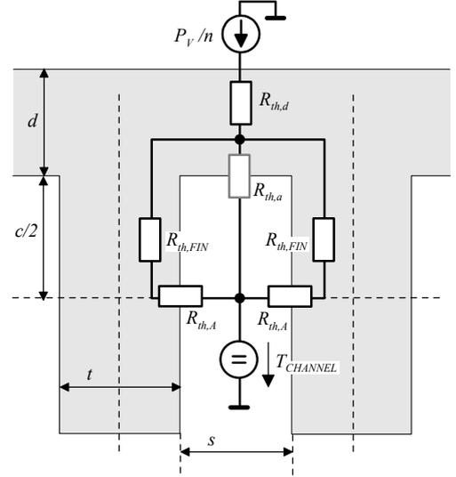
**Fig.3:** Thermal network describing (stationary) heat conduction between heat sink base plate and the air in the channel (temperature  $T_{CHANNEL}$ ).
