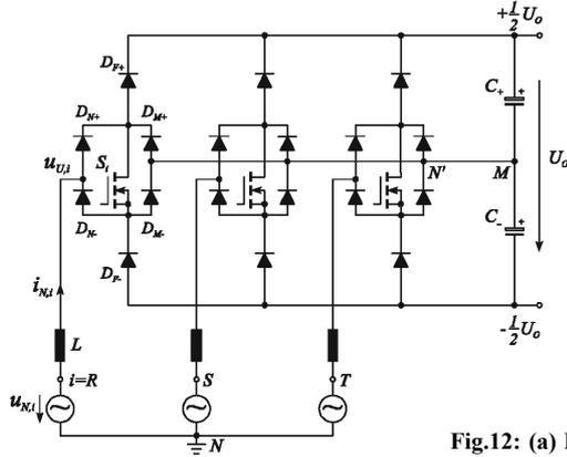
**Fig.12:** (a) Power circuit of the Vienna Rectifier with input voltage amplitude  $327V$ , DC output voltage  $800V$ , output power  $10kW$  and switching frequency  $500kHz$ . (b) Power module realizing one bridge-leg of the three-phase Vienna Rectifier employing SiC-free-wheeling diodes ( $D_F$ ), a CoolMOS power transistor (S), and Si-diodes ( $D_N, D_M$ ).
