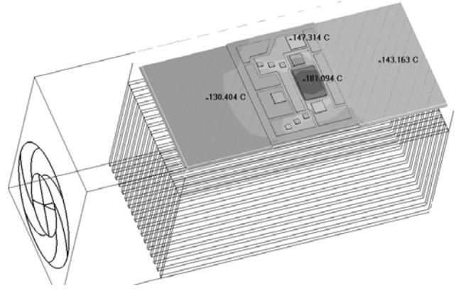
**Fig.14:** Details of the stationary temperature distribution inside one power module specified in Fig.12(b) employing the cooling system “Type (B)” (Fig.5) derived from a 3D-FEM CFD simulation (ICEPAK). The power switch realized by a CoolMOS is by far the hottest chip ( $180^\circ\text{C}$ ). Therefore, the critical junction temperature of the converter design is always that of the transistor.
