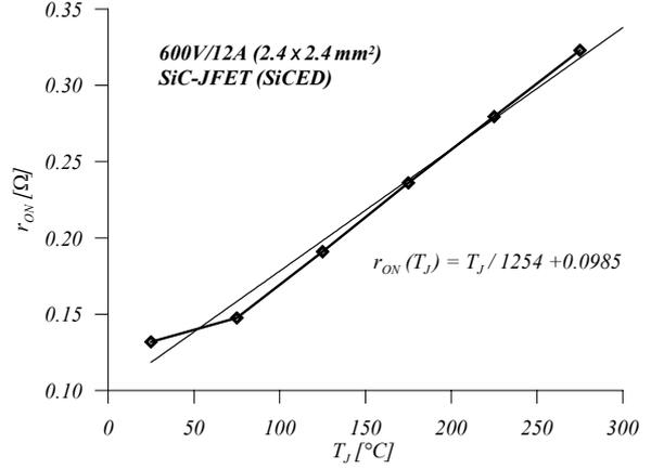
**Fig.10:** Temperature dependency of the on-resistance  $R_{DS(on)}$  of the  $600V/12A$  SiC-JFET transistor (chip size  $2.4 \times 2.4 mm^2$ ) from SiCED [15].
