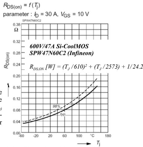
**Fig.7:** Temperature dependency of the on-resistance  $R_{DS(on)}$  of a 600V/47A Si-CoolMOS power transistor [9].
