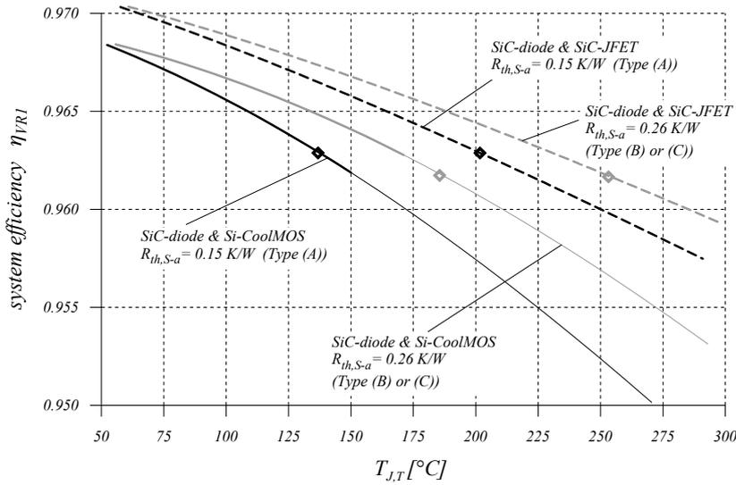
**Fig.15:** Converter system efficiency dependent on the transistor junction temperature for two different kind of heat sinks characterized by their thermal resistance  $R_{th,S-a}$  (Tab.2) and two different kind of semiconductors (Tab.4 vs. Tab.5). With higher temperatures the system efficiency generally decreases. The four square symbols on the curves indicate operating points where  $P_{OUT} = 10kW$  can be achieved.
