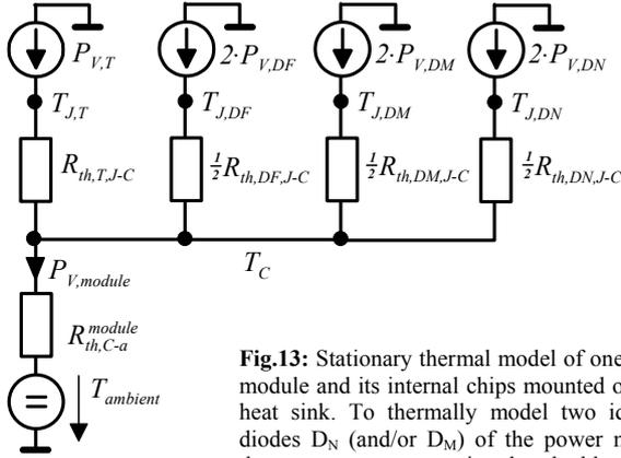
**Fig.13:** Stationary thermal model of one power module and its internal chips mounted onto the heat sink. To thermally model two identical diodes  $D_N$  (and/or  $D_M$ ) of the power module, the current source emits the double current (power loss of two diodes) but assumes half of the thermal resistance to calculate correctly both the chip junction temperature and the total output power of the module.
