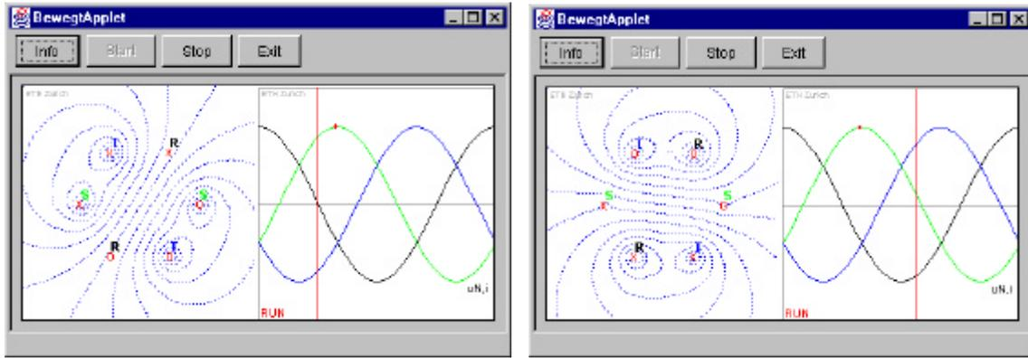
**Fig. 7:** The symbols "x" and "o" shown in red do denote impressed currents of opposite directions in conductors of infinite length oriented perpendicular to the drawing plane. Always two conductors of equal denomination can be considered to form a phase winding.
