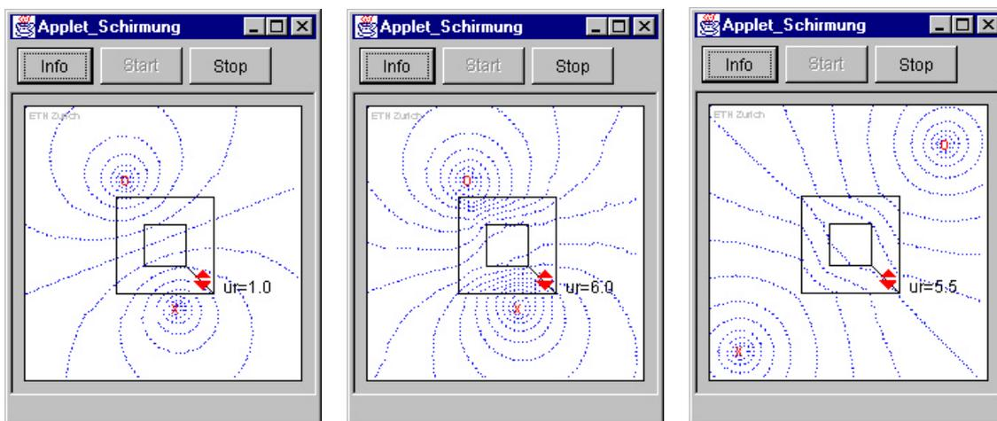
**Fig. 2:** By changing the permeability of the rectangular magnetic material one can experience how the magnetic flux lines are influenced by permeable material.
