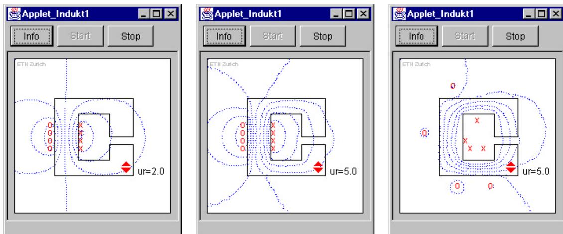
Fig. 5: By changing the permeability of the magnetic core one can see how the magnetic flux distribution is influenced by magnetic material. The shape of the magnetic material is typical for an inductor.
