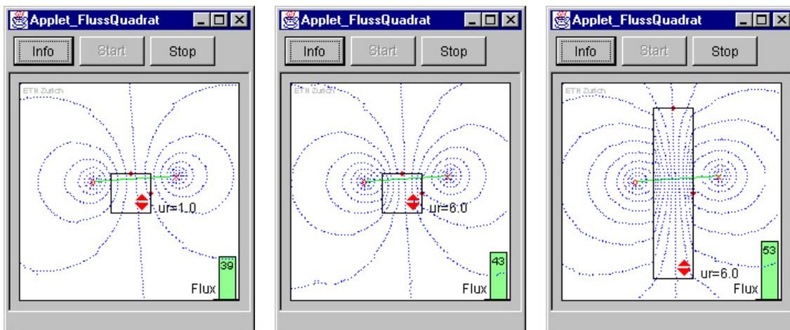
**Fig. 3:** By changing the size, shape and permeability of the rectangular shaped magnetic material one can see how the magnetic flux lines are influenced by material with magnetic properties. Furthermore, the influence of the magnetic material and of the geometry on the magnetic flux is shown.
