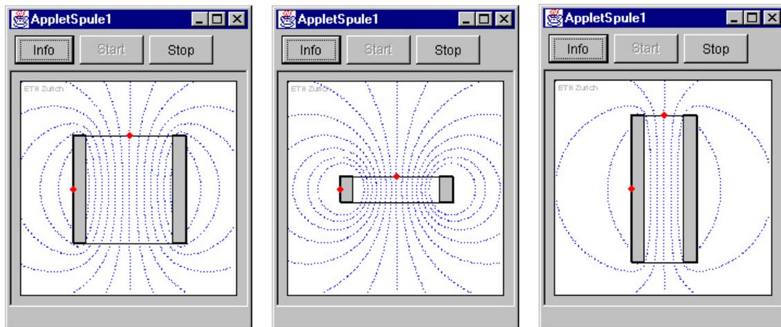
Fig. 4: The dimensions of the coil can be changed by dragging the red dots with the mouse. The applet shows the magnetic flux lines. While changing the dimensions of the inductor the value of the ampere-turns remains constant.
