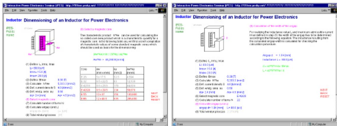
**Fig. 6:** The applet shows an intuitive and user-friendly step-by-step approach for dimensioning an inductor for a power electronics converter. The calculations are based on simplified analytical equations as given in the applet. Stray fields are neglected.
