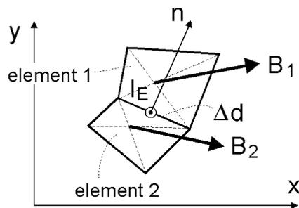
**Fig. 8:** Magnetic material modeled with two elements. The elementary current  $I_E$  between the two elements 1 and 2 is calculated according to equation (11).
