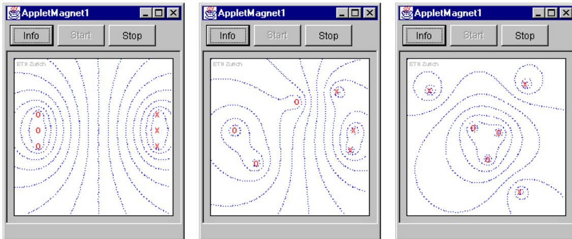
**Fig. 1:** Magnetic flux lines of impressed currents of opposite directions in conductors of infinite length oriented perpendicular to the drawing plane. The positions of the current carrying conductors can be changed with the mouse.
