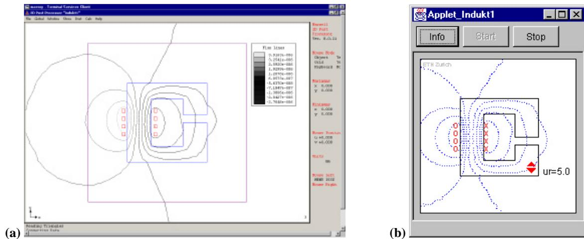
**Fig. 9:** (a) Computation of the flux lines for  $\mu_r = 5$  using Maxwell 2D; (b) computation of the flux lines ( $\mu_r = 5$ ) by the Java applet.
