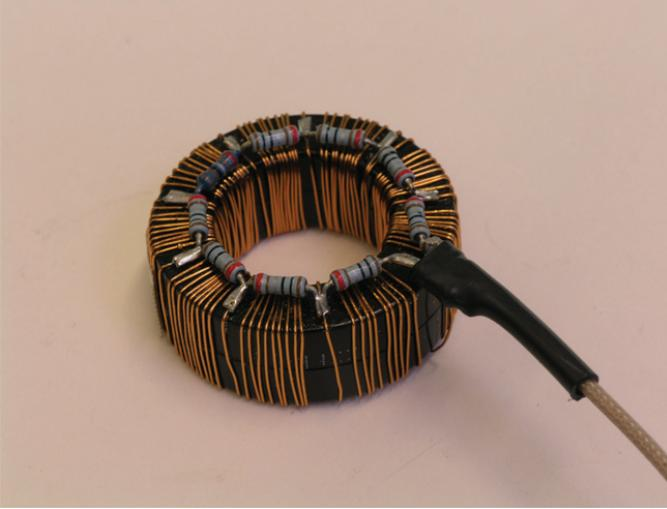
**Figure 6.10:** The damping effect of the resistors across the winding's turns is equivalent to the damping effect of the core resistance in wound ferrite components.
