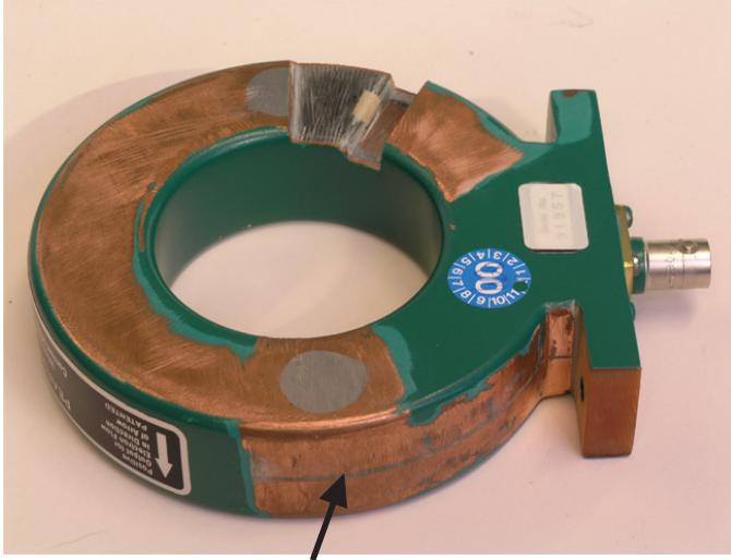
**Figure 6.16:** The screen of a Pearson current transformer is gapped, to avoid a magnetic short circuit.
