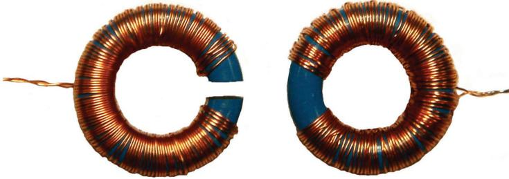
**Figure 5.10:** Prototypes of the broadband DC-CT. Ungapped toroids were used for empirical characterization.
