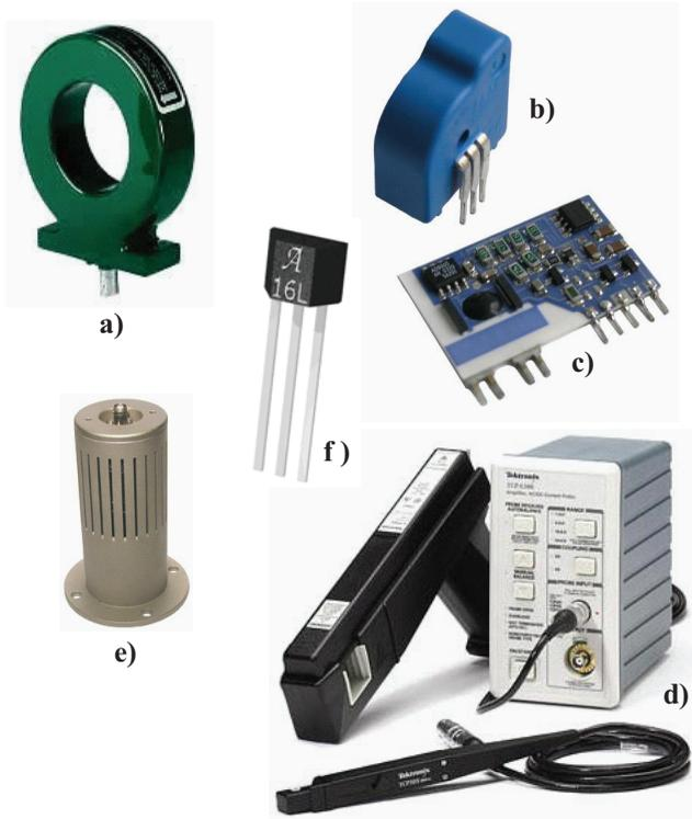
**Figure 1.12:** Commercial current sensors: a) Current transformer, 20 MHz; b) Closed-loop, DC to 200 kHz current sensor; c) DC to 100 kHz magnetostrictive sensor; d) zero-flux, DC to 100 MHz current probe; e) 100 MHz shunt; f) DC to 10 kHz, Hall-effect element.
