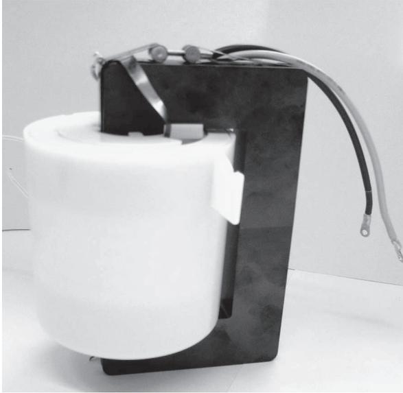
**Figure 6.2:** Photograph of a high-voltage transformer.
