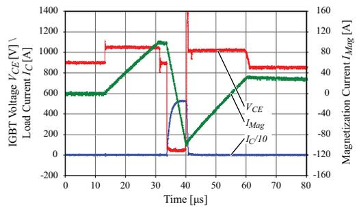
Fig. 9: Symmetric flux swing, where  $T_{Premag} \approx T_{Demag}$
