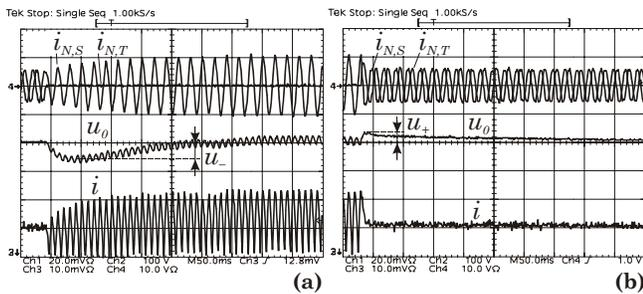
**Fig. 7:** Time behavior of the output voltage for the disconnection (a) and for the reconnection (b) of mains phase  $T$ . Operating parameters, voltage and current scales as in Fig. 6.
