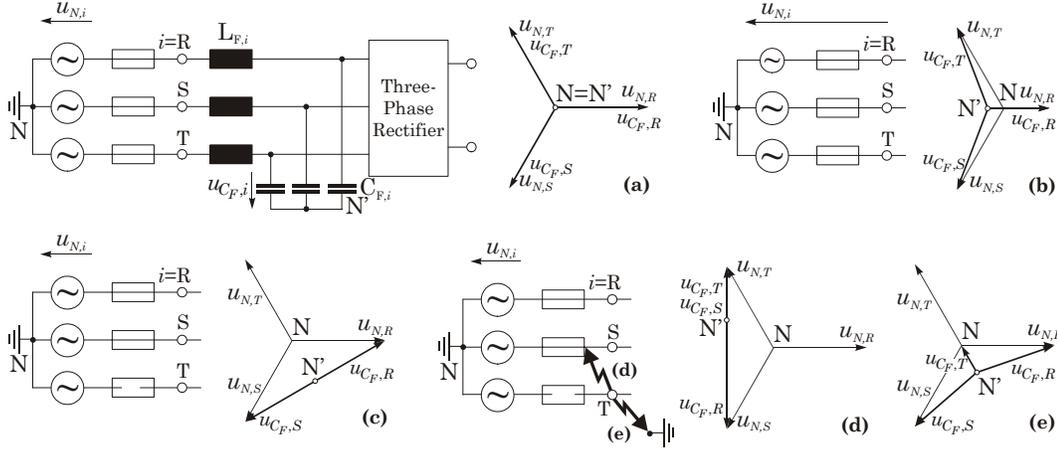
**Fig. 4:** Mains phase conditions and corresponding phasor diagrams of mains phase voltages  $u_{N,i}$  and input filter capacitor voltages  $u_{C_F,i}$ . (a): symmetric mains condition, (b): mains phase voltage unbalance:  $u_{N,R}$  is 50% smaller than for symmetric conditions. (c)-(e): Two phase operation, (c): loss of phase  $T$ , (d): short circuit between phases  $S$  and  $T$ , and (e): earth fault in phase  $T$ .
