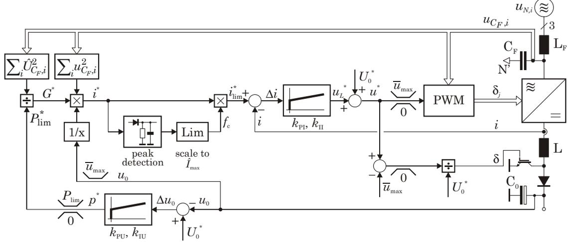
**Fig. 3:** Control structure guaranteeing unity power factor operation under heavily unbalanced mains.
