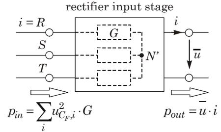
**Fig. 2:** Equivalent circuit of the input stage of the three-phase rectifier system showing the balance of input and output power.
