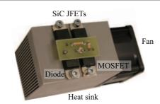
Fig. 13. High-voltage SiC switch built with discrete components.
