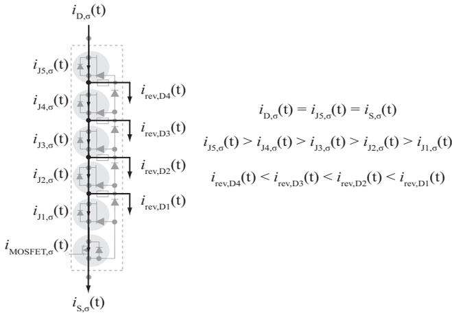
Figure 13: Leakage current distribution in the SiC HV Switch.
