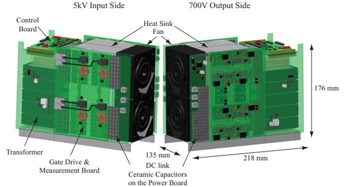
Figure 18: 3D-model of the DAB dc-dc converter.
