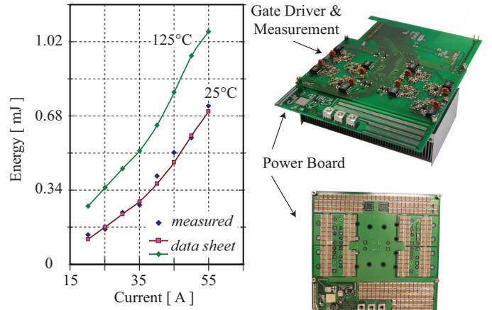
Figure 4: Measurement of the IGBT turn-off energy losses @350 V with the three level converter prototype.
