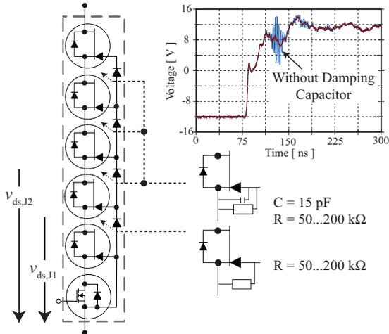
Figure 14: Additional resistors and capacitors guarantee a well defined leakage current and damp oscillations in the gate-source voltage (measured at a power supply voltage of 2 kV).
