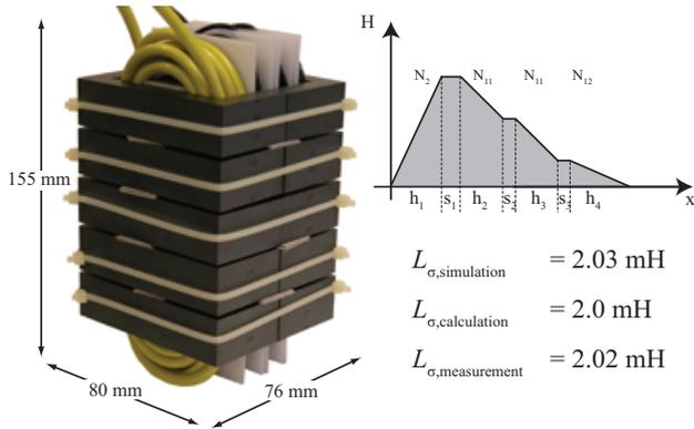
Figure 8: 5 kV/50 kHz transformer prototype with a leakage inductance of  $L_\sigma = 2.02$  mH and distribution of the magnetic field between the primary and secondary winding.
