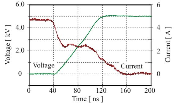
Figure 16: Turn off behaviour of the HV SiC JFET cascode at 5 kV.
