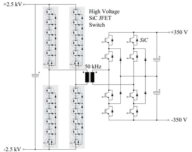
Figure 2: 25 kW (5 kV/700 V), 50 kHz DAB DC-DC converter based on high voltage SiC JFETs.
