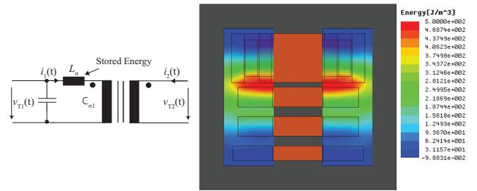
Figure 9: 3D FEM simulation of the the energy density in a cut plane through one of the cores. There, balanced magnetomotive forces  $N_1 I_1 = N_2 I_2$  have been assumed, so that the magnetic field only represents the energy stored in the leakage inductance.
