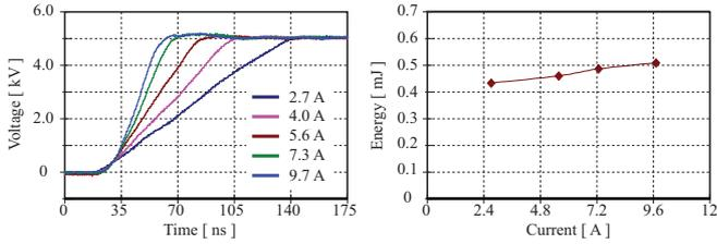
Figure 17: Voltage waveforms during turn off for different load currents and the “turn off” energy. This energy is stored in the parasitic capacitances, what results in negligible turn off losses.
