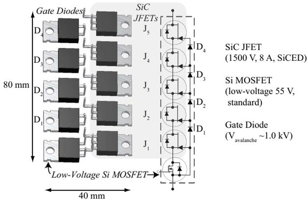
Figure 3: A SiC JFET cascode consists of five SiC JFETs, a low-voltage Si MOSFET and four gate diodes.
