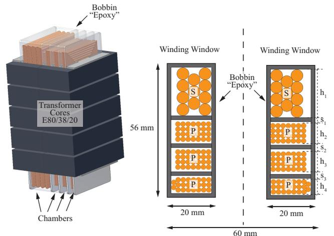
Figure 7: 3D-model of the 5 kV, 50 kHz transformer made of five parallel EE80/38/20 cores with a possible winding arrangement.
