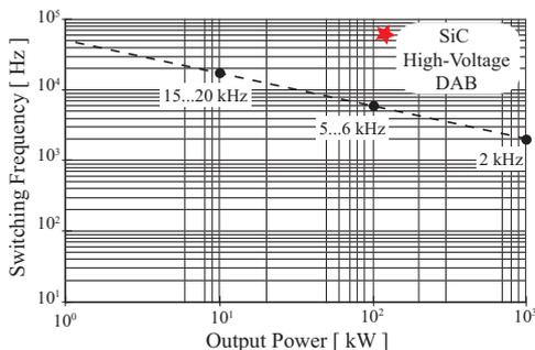
Figure 1: Common converter operating frequency versus output power with conventional semiconductors. The star marks the operating point of the DAB based on SiC-JFET devices presented in this paper.
