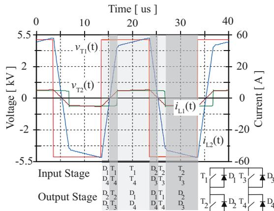
Figure 6: DAB waveforms for phase-shift modulation at  $V_1=5$  kV,  $V_2=700$  V and  $P_{out}=25$  kW. At the bottom the semiconductors, which conduct in the respective interval, are shown.
