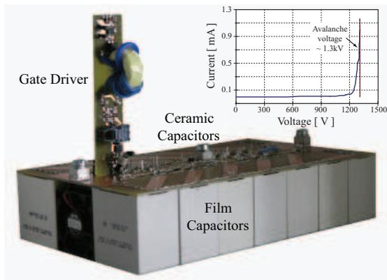
Figure 10: Test bench consisting of a half bridge with two switches consisting of a MOSFET and five cascaded JFETs for experimental investigation of the switching behaviour up to 5kV. On the right hand side the avalanche behaviour of the voltage balancing diodes is shown.
