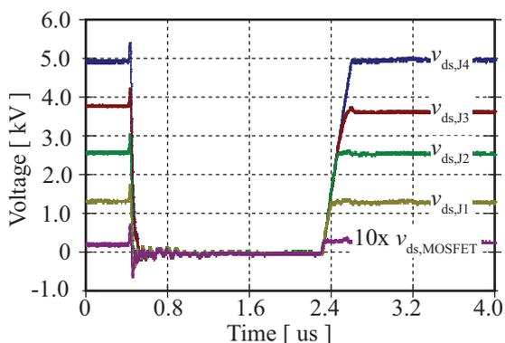
Figure 11: Voltage distribution across the SiC JFET cascade caused by the avalanche voltage of the gate diodes. The measurement are made with DA1855A amplifier from LeCroy.
