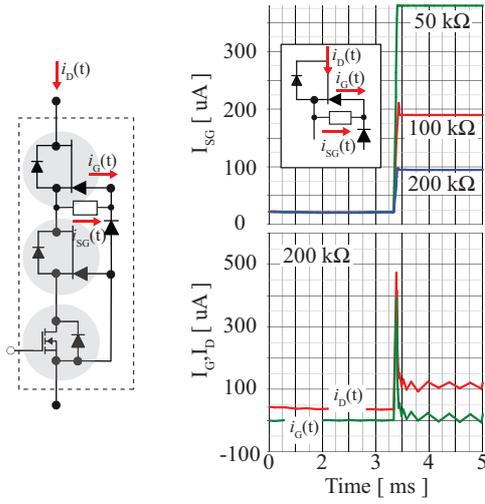
Figure 12: Depending on the gate-source resistor, the leakage current and therefore the operating point of the avalanche rated diode can be controlled. Simulations are made with SIMetrix and are based on the SiC JFET model from SiCED.
