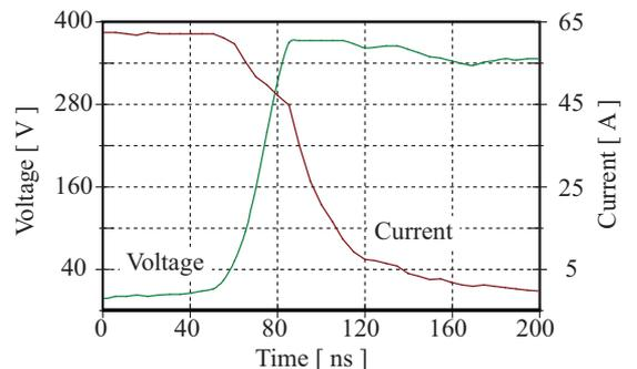
Figure 5: Turn-off waveforms of the APT40GP60B IGBTs utilised in three level converter at a voltage of 350 V and a current of 62 A.
