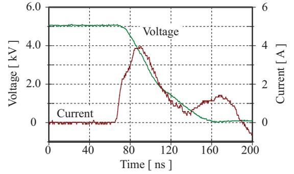
Figure 15: Turn on behaviour of the HV SiC JFET cascode at 5 kV.
