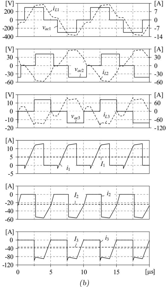
**Figure 3.11:** Simulation of steady-state waveforms for operating point *A* (a) and *B* (b) in Figure 3.10. The current magnitudes and the voltage and current phase displacements of the operating point *B* are higher than those of operating point *A*, resulting in significantly higher losses (continued).
