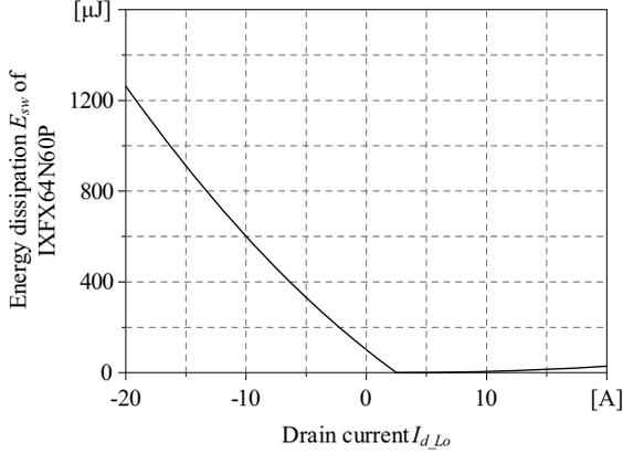
**Figure 3.8:** Dependency of the energy dissipation  $E_{sw}$  of a MOSFET IXFX64N60P employed in a bridge leg on the drain current  $I_{dLo}$ . The drain current  $I_{dLo}$  is positive when the current in the MOSFET  $S_{Lo}$  is diverted to the body diode  $D_{Hi}$ , i.e. when zero-voltage-switching occurs, and is negative when the current in the body diode  $D_{Lo}$  is diverted to the MOSFET  $S_{Hi}$ , i.e. for hard-switching.
