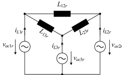
**Figure 2.13:**  $\Delta$ -type primary-referred equivalent circuit of the proposed topology (cf. Figure 2.1).
