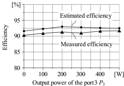
**Figure 3.16:** Comparison of the estimated and the measured total system efficiency for different output power levels of port 3 with the constant output power of port 2, i.e.  $P_2 = -1$  kW).
