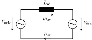
**Figure 2.7:** Simplified primary-referred equivalent circuit for studying the energy transfer between two ports when the third port is left open.
