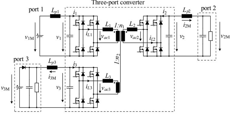
**Figure 5.1:** Implemented three-port system. Port 1 is connected with a voltage source; port 2 is connected with a RC Load and port 3 is connected with a RC load in parallel to a voltage source.
