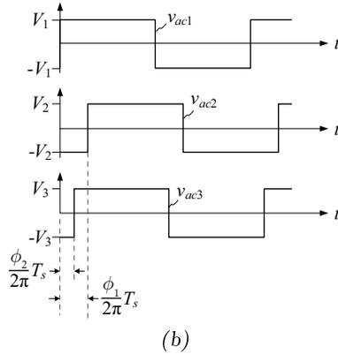
**Figure 2.4:** (a) Simplified equivalent circuit of the proposed topology (cf. Figure 2.1); (b) Idealized high-frequency voltages  $v_{ac1}$ ,  $v_{ac2}$  and  $v_{ac3}$ , where  $\phi_1$  and  $\phi_2$  denote the phase displacement of  $v_{ac1}$  and  $v_{ac2}$  and  $v_{ac1}$  and  $v_{ac3}$ , respectively.
