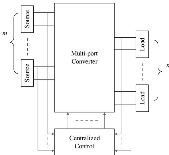
**Figure 1.3:** Block diagram of a power electronic system with a multi-port converter.
