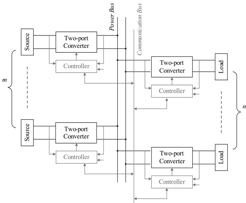
**Figure 1.2:** Block diagram of a power electronic system with various two-port converters.
