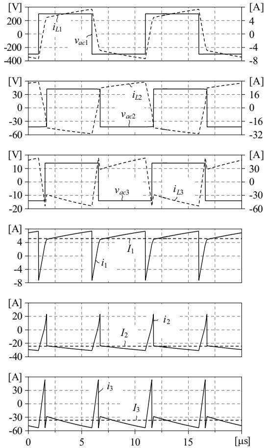
**Figure 2.17:** Steady-state simulation waveforms for operating point  $a$  ( $\phi_{1a} = 0.488$ ,  $\phi_{2a} = 0.381$ ), resulting in  $P_1 = 1.5$  kW,  $P_2 = -1.0$  kW and  $P_3 = -0.5$  kW.
