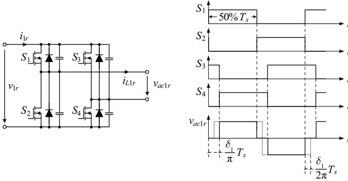
**Figure 3.2:** Idealized gate signals waveforms and high-frequency voltage waveform  $v_{ac1r}$  with a time span of the positive/negative voltage pulse  $(1/2 - \delta_1/\pi)T_s$ .
