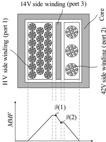
**Figure 3.9:** Transformer winding arrangement and associated m.m.f. diagram for operation in optimum operating point *A* (cf. Figure 3.10).
