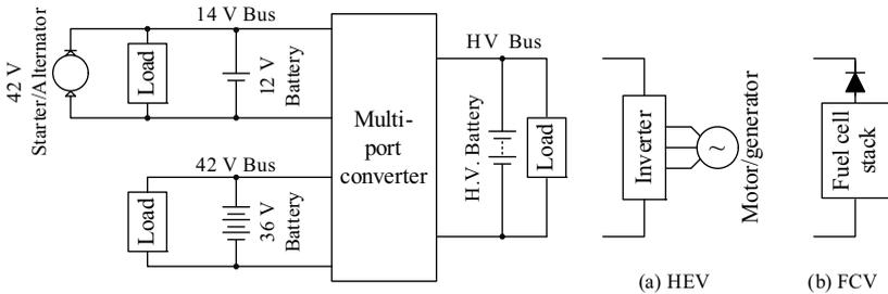
**Figure 1.9:** A multi-port converter interconnecting 14 V/42 V/HV bus in HEVs and FCVs.
