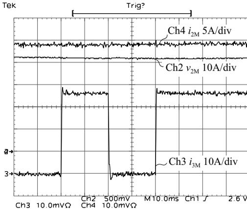
**Figure 5.5:** Measured dynamic system behavior with a pulsating current reference signal  $I_{3M\_ref} = 0$  A, = 35.7 A ( $P_{3\_ref} = -500$  W), = 0 A and = 35.7 A and a constant voltage reference signal  $V_{2M\_ref} = 42$  V ( $P_{2\_ref} = -1$  kW).
