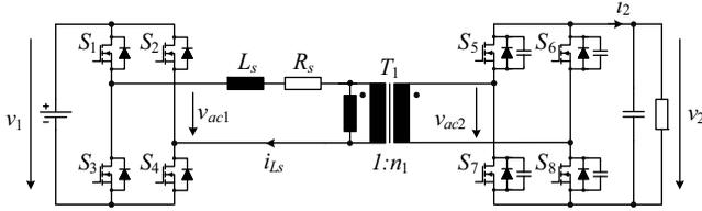
**Figure 4.2:** DAB DC-DC converter with a battery and a RC load.
