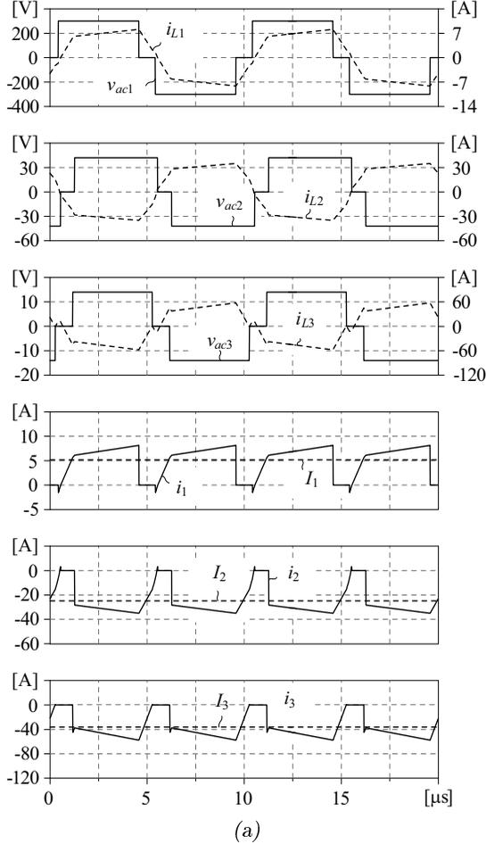
**Figure 3.11:** Simulation of steady-state waveforms for operating point *A* (a) and *B* (b) in Figure 3.10. The current magnitudes and the voltage and current phase displacements of the operating point *B* are higher than those of operating point *A*, resulting in significantly higher losses.
