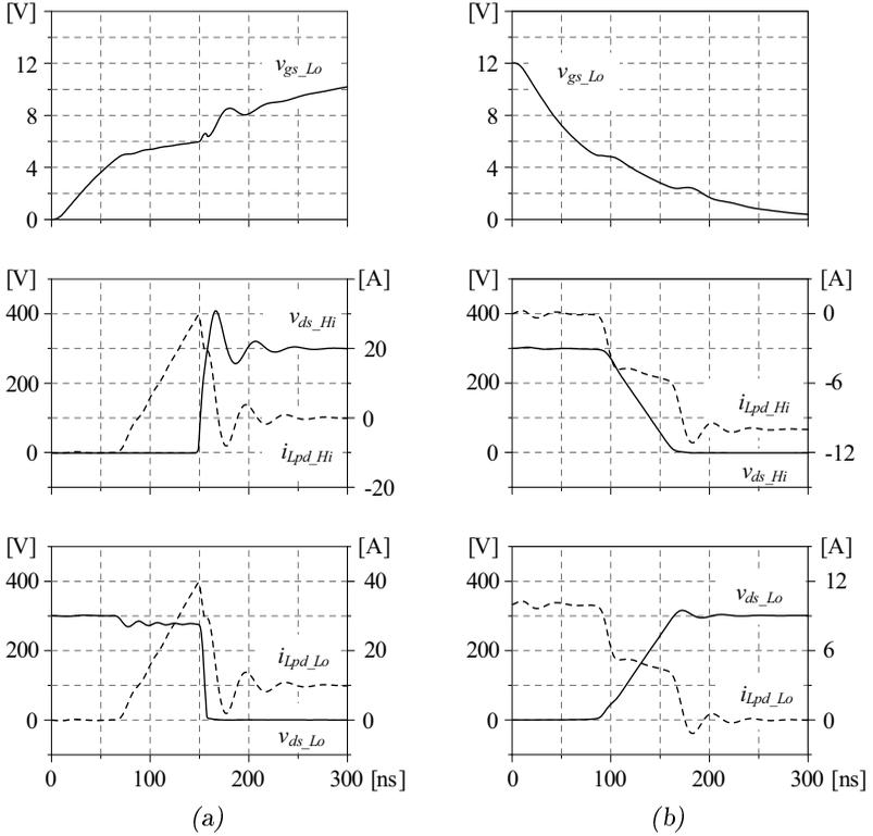
**Figure 3.7:** (a) Turn-on and (b) turn-off waveforms of a bridge leg employing MOSFETs IXFX64N60P based on numerical calculations.
