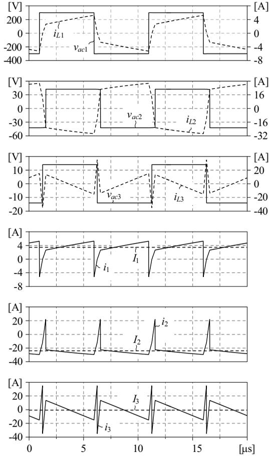
**Figure 2.18:** Steady-state simulation waveforms for operating point  $b$  ( $\phi_{1b} = 0.369$ ,  $\phi_{2b} = 0.178$ ), resulting in  $P_1 = 1.0$  kW,  $P_2 = -1.0$  kW and  $P_3 = 0$  kW.
