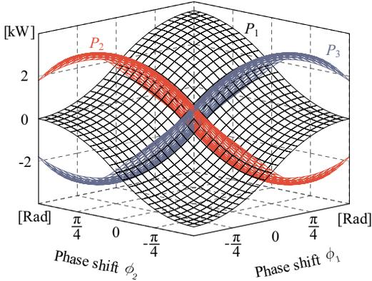
**Figure 2.15:** Dependency of the input/output active power,  $P_1$ ,  $P_2$  and  $P_3$ , on the phase shift angles  $\phi_1$  and  $\phi_2$ ; parameters as given in Table 2.2.
