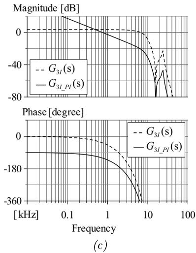
**Figure 5.4:** Bode plots of the open loop gains of the three-port converter and bode plots of the loop gains with PI controllers: (a) current control loop  $i_{2M}$ ; (b) voltage control loop  $v_{2M}$ ; (c) current control loop  $i_{3M}$  (continued).
