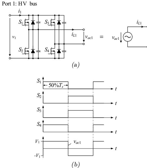
**Figure 2.3:** (a) High-frequency voltage source representing the full-bridge unit and the associated voltage bus; (b) Idealized gate signals waveforms and high-frequency voltage waveform  $v_{ac1}$ , which is determined by the pattern of the switch gate signals and the port voltage level  $V_1$ .
