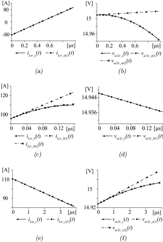
**Figure 4.4:** (a)-(g) Comparison of the actual state variable instantaneous waveforms with their first- and/or second-order approximations. The circuit and operating parameters are given in Table 4.1 as for Model (d).
