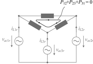
**Figure 3.4:** Zero active circulating power, i.e.  $P_{12} + P_{23} + P_{31} = 0$ .
