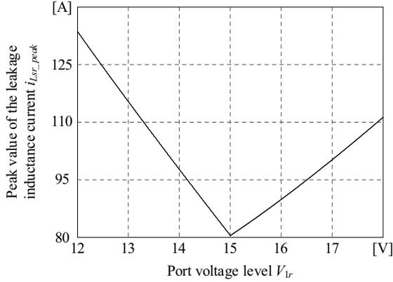
**Figure 2.12:** Peak value of the inductance current  $i_{Lsr\_peak}$  within one switching cycle versus voltage level  $V_{1r}$  when transferring a constant power  $P_{12} = 1$  kW; other parameters as given in Table 2.1.
