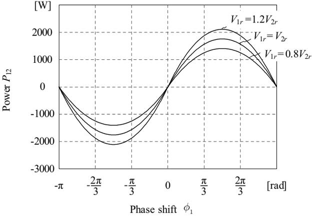
**Figure 2.9:** Power  $P_{12}$  versus phase shift angle  $\phi_1$  with parameters as given in Table 2.1.
