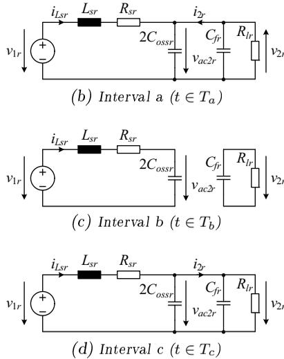
**Figure 4.3:** (a) Idealized primary-referred time behaviors of the terminal voltages  $v_{ac1r}$  and  $v_{ac2r}$  of the intermediate circuit, leakage inductance current  $i_{Lsr}$ , output current  $i_{2r}$  and output voltage  $v_{2r}$  for steady-state operation; the waveforms are shown for one switching cycle  $T_s = 2T_{samp}$ . (b)-(d) Primary-referred equivalent circuits for three switching states (continued).
