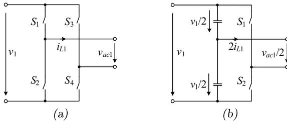
**Figure 2.2:** Circuit schematic of (a) full-bridge unit and (b) half-bridge unit.
