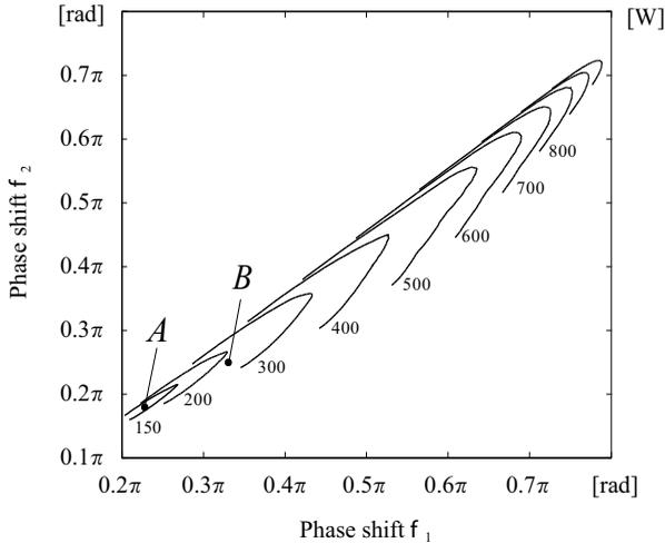
**Figure 3.10:** Overall converter losses in the whole admissible operating area *Area A* in dependency on  $\phi_1$  and  $\phi_2$ ; operating point *A* results in minimum overall converter losses. Operating parameters and circuit parameters as for Figure 3.5.
