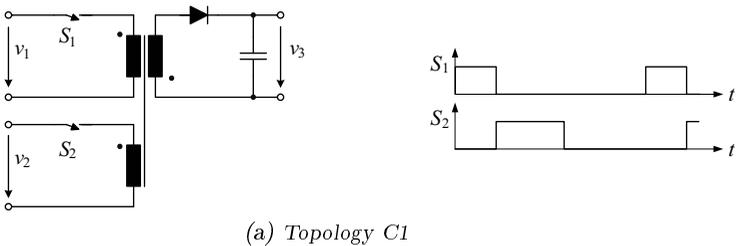
**Figure 1.12:** (a)-(e) Different fully isolated multi-port topologies and related gate signals of the switches.
