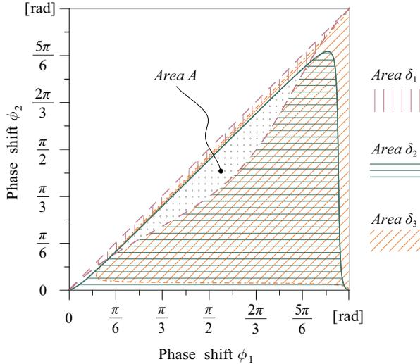
**Figure 3.5:** Operating area  $A$ , i.e. admissible range of phase shift angle  $\phi_1$  and phase shift angle  $\phi_2$ , for  $P_1 = 1.5$  kW,  $P_2 = -1.0$  kW,  $P_3 = -0.5$  kW, and zero circulating power; other parameters as given in Table 2.2.
