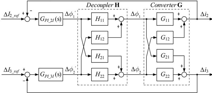
**Figure 5.2:** Block diagram of the control system with the decoupling network.  $\mathbf{G}$  is the small signal transfer function matrix of the three-port converter and  $\mathbf{H}$  denotes the transfer function matrix of the decoupling network.
