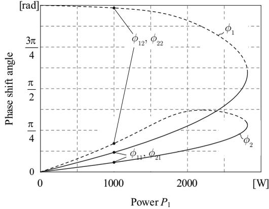
**Figure 2.16:** Phase shift angles  $\phi_1$  and  $\phi_2$  for achieving  $P_1 = -P_2 = 1$  kW and  $P_3 = 0$  W; parameters as given in Table 2.2.
