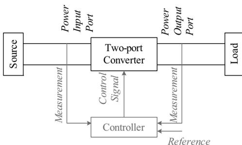
**Figure 1.1:** Block diagram of a power electronic system with a source and a load.
