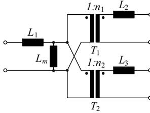
**Figure 2.5:** Simplified equivalent circuit of the three-winding transformer  $T_r$  [79].
