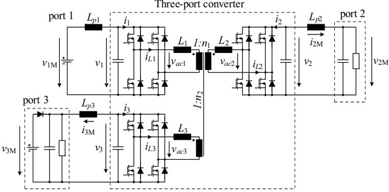
**Figure 3.13:** Implemented three-port system, where three LC filters connect the ports to the sources or loads.
