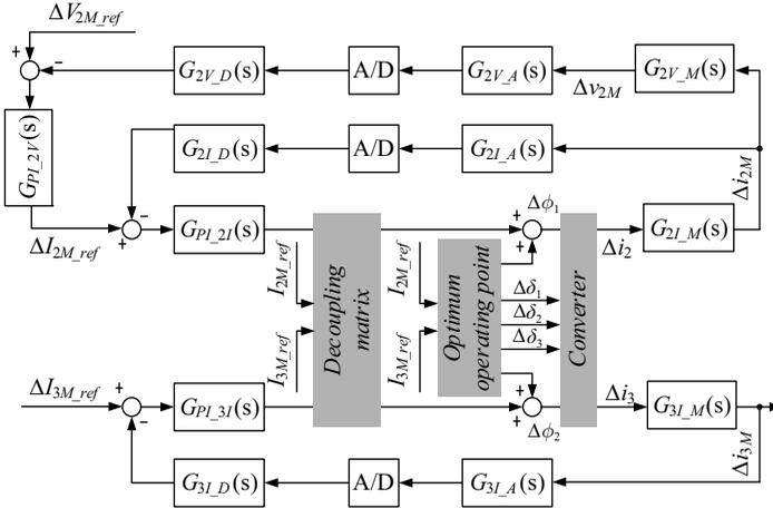
**Figure 5.3:** Block diagram of the control loops of the implemented three-port converter.
