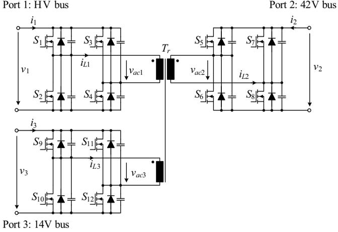
**Figure 2.1:** Proposed isolated three-port bidirectional converter topology, where high frequency linking of the full-bridge units is realized via a single transformer  $T_r$ .
