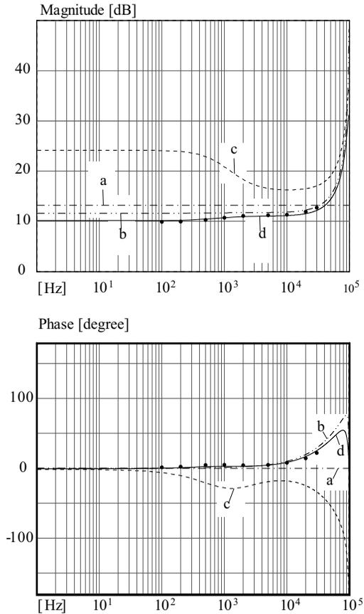
**Figure 4.7:** Control-to-output-current frequency responses of the DAB DC-DC converter as predicted by Models (a), (b), (c) and (d). Dots represent the detailed switching model simulation results obtained using SIMPLORER.
