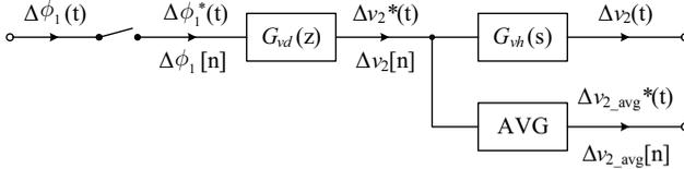
**Figure 4.1:** Small signal system for the phase-shift bidirectional DC-DC converter.
