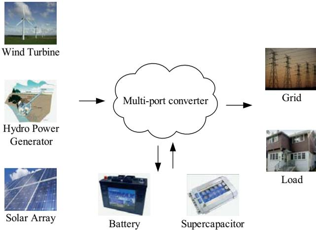
**Figure 1.5:** Multi-port converter utilization in renewable energy generation systems.
