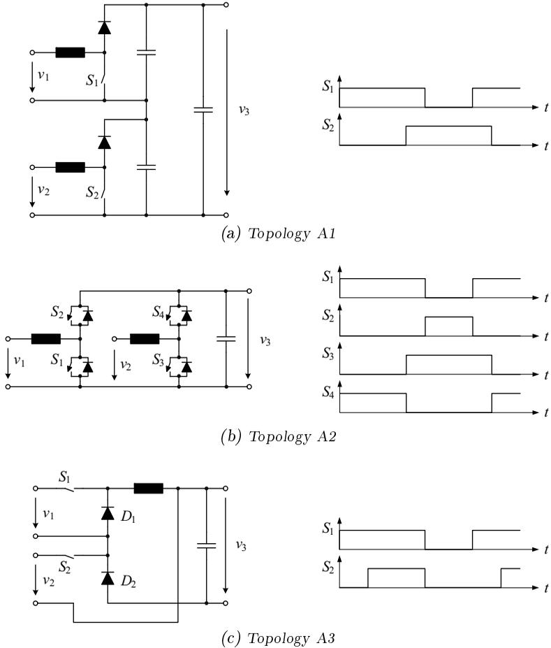
**Figure 1.10:** (a)-(f) Different non-isolated multi-port topologies and related gate signals of the switches.
