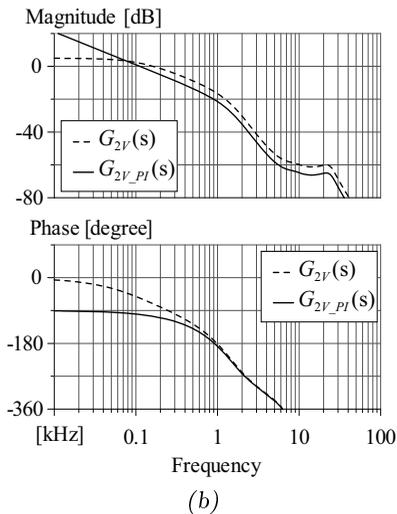
**Figure 5.4:** Bode plots of the open loop gains of the three-port converter and bode plots of the loop gains with PI controllers: (a) current loop controlling  $i_{2M}$ ; (b) voltage loop controlling  $v_{2M}$ ; (c) current loop controlling  $i_{3M}$ .
