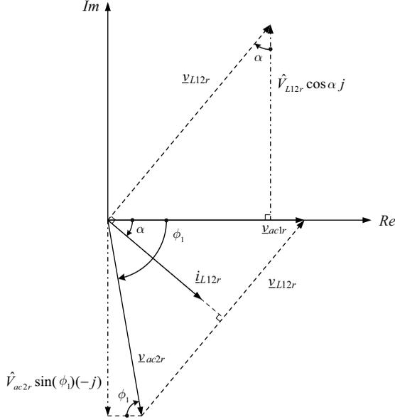
**Figure 3.3:** Phasor diagram for the converter voltages and currents.
