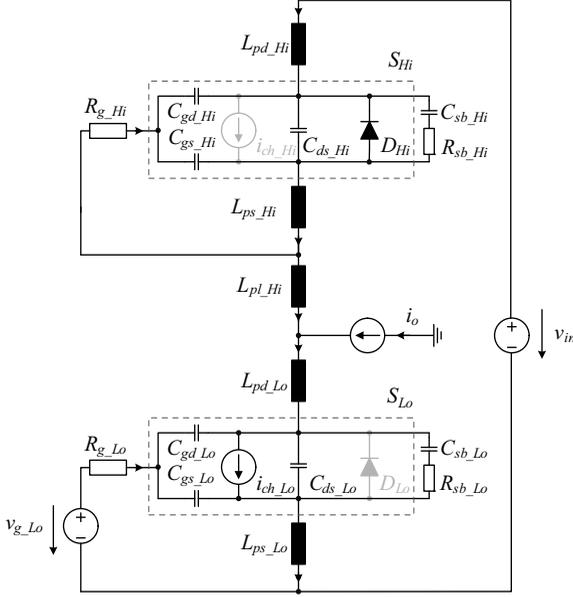
**Figure 3.6:** Equivalent circuit of the test setup within the commutation interval when the current in MOSFET  $S_{Lo}$  is diverted to the body diode  $D_{Hi}$ . The suffixes  $_{Hi}$  and  $_{Lo}$  denominate the components associated to the upper MOSFET  $S_{Hi}$  and the lower MOSFET  $S_{Lo}$ .
