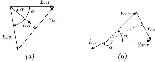
**Figure 2.10:** Fundamental phasor diagram of the voltages and currents of the two-port circuit (a)  $\phi_1 > 0$  and (b)  $\phi_1 < 0$ .
