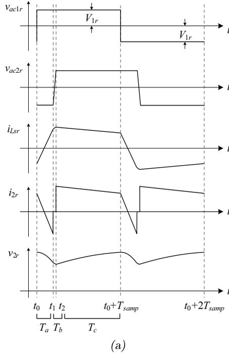
**Figure 4.3:** (a) Idealized primary-referred time behaviors of the terminal voltages  $v_{ac1r}$  and  $v_{ac2r}$  of the intermediate circuit, leakage inductance current  $i_{Lsr}$ , output current  $i_{2r}$  and output voltage  $v_{2r}$  for steady-state operation; the waveforms are shown for one switching cycle  $T_s = 2T_{samp}$ . (b)-(d) Primary-referred equivalent circuits for three switching states.
