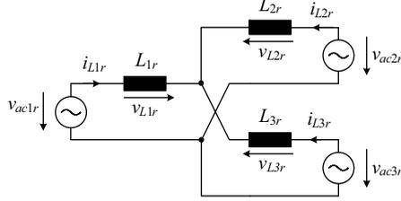
**Figure 2.6:** Simplified Y-type equivalent circuit of the proposed topology (cf. Figure 2.1) referred to the transformer primary side.
