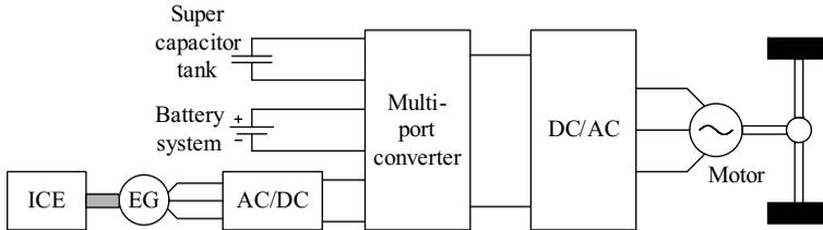
**Figure 1.7:** Hybrid propulsion system proposed in [53].
