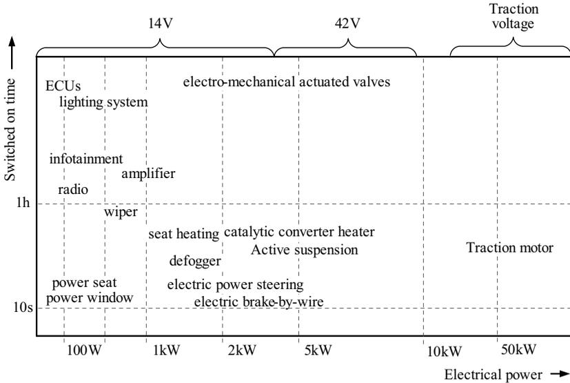
**Figure 1.8:** Power requirement for existing and prospective electrical systems in HEVs and FCVs [62].
