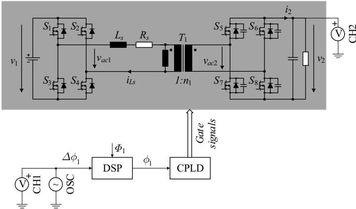
**Figure 4.6:** Experimental setup for measuring the loop frequency response.
