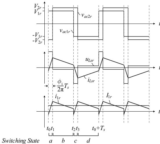
**Figure 2.8:** Idealized voltage and current waveforms of the two-port circuit for  $v_{ac1r}$  leading  $v_{ac2r}$ .
