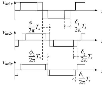
**Figure 3.1:** Definition of phase displacements and duty cycles of the full-bridge unit output voltages  $v_{ac1r}$ ,  $v_{ac2r}$  and  $v_{ac3r}$ .
