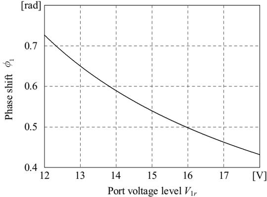
**Figure 2.11:** Dependency of the phase shift angle  $\phi_1$  on the voltage level  $V_{1r}$  for transferring a constant amount of power  $P_{12} = 1$  kW; other parameters as given in Table 2.1.
