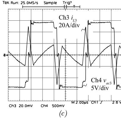
**Figure 3.15:** Measured waveforms, showing the voltages between the phase leg midpoints of the full-bridge units and the related transformer winding currents, for the optimum operating point with  $P_2 = -1$  kW and  $P_3 = 0$  W (continued).
