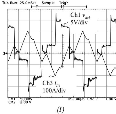
**Figure 3.14:** Measured waveforms, showing the voltages between the phase leg midpoints of the full-bridge units and the input current of each winding. (a), (b), (c) are related to operating point *A* and (d), (e), (f) to operating point *B* (cf. Figure 3.10) with  $P_2 = -1$  kW and  $P_3 = -500$  W. One has to note, that operating point *A* in general is characterized by the lowest system losses (continued).
