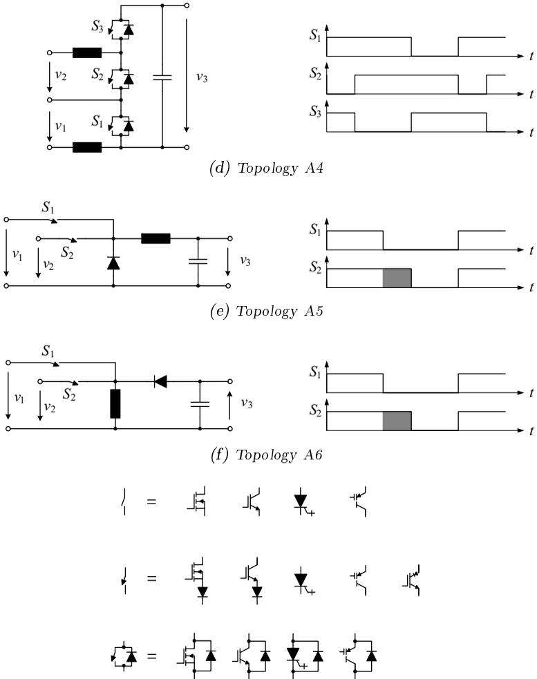
**Figure 1.10:** (a)-(f) Different non-isolated multi-port topologies and related gate signals of the switches (continued).
