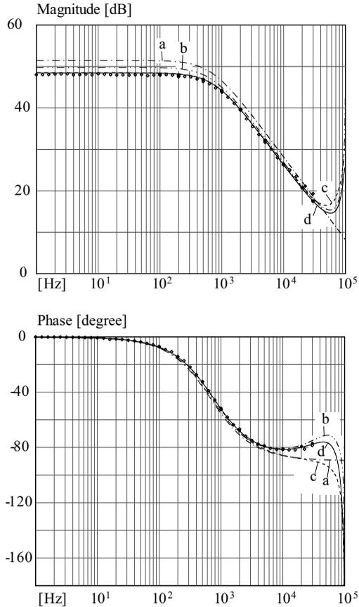
**Figure 4.8:** Control-to-output-voltage frequency responses of the DAB DC-DC converter as predicted by Models (a), (b), (c) and (d). Dots and rhombuses represent the detailed switching model simulation results obtained using SIMPLORER and the measured results obtained using a Venable Model 350 frequency response analyzer, respectively.
