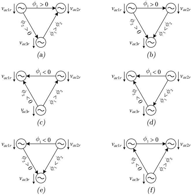
**Figure 2.14:** Equivalent circuit for studying the power flow between the three ports. The direction of power flow is only determined by the phase shift angles  $\phi_1$  and  $\phi_2$ , not by the voltage levels  $V_{1r}$ ,  $V_{2r}$  and  $V_{3r}$ .
