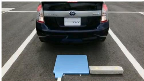
▲ IPT charging station with parking guides
