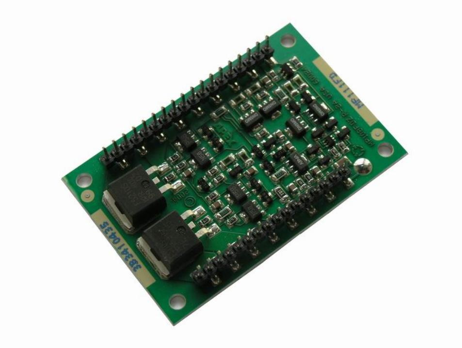
Figure 5.6: APEX power operational power amplifier MP111FD. The dimensions are 41.4 mm x 63.2 mm x 11.5mm.
