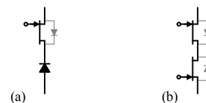
Fig. 3. Replacement of the bridge-leg series diode (a) with a SiC JFET (b).
