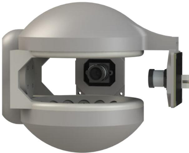
**Fig. 3.12:** The demonstrator used to verify the developed methods. It uses 72 transducers operating at 40kHz and two cameras for the position and orientation detection.
