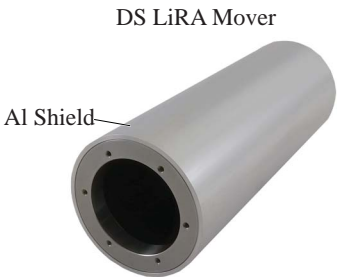
Fig. 8.30: DS LiRA mover with the aluminum shields from the inner and outer sides.
