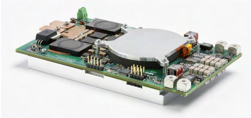
**Fig. 1.12:** Hardware demonstrator of the 3.6 kW 500 V/500 V/15 V three-port DC/DC resonant converter with a phase-shifted full-bridge equivalent circuit in the LV port.
