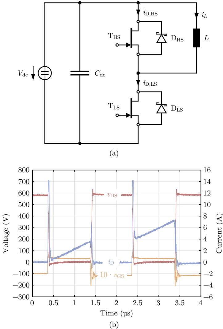
Figure 8.1: (a) Test setup for the validation of the gate driver circuit: Half-bridge connection of two 1200 V 40 A normally-off SiC JFETs with antiparallel freewheeling diodes (SiC Schottky Barrier Diodes Infineon IDH15S120 [94]) and an inductive load. (b) Time behavior of the drain current, drain-source and gate-source voltage of the low-side switch.
