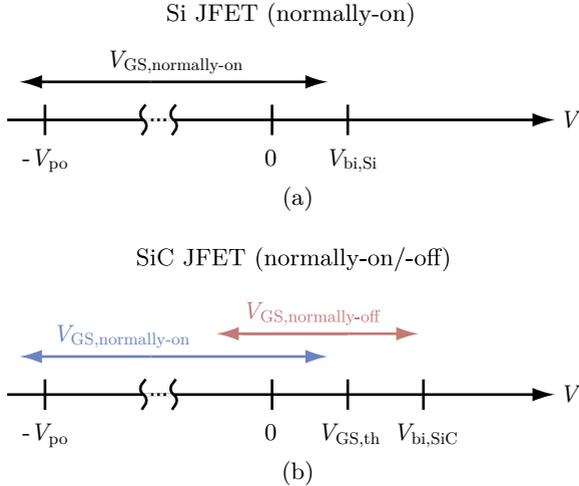
Figure 2.1: Gate-source voltage ranges for (a) normally-on JFETs in Si as well as (b) normally-on and -off JFETs in SiC.
