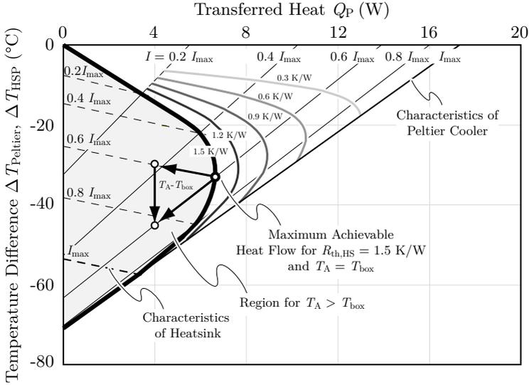
Figure 5.8: Characteristic curves of Peltier cooler (solid lines) and heat sink for the Peltier cooler (dashed lines). Intersections (thick solid line) mark the possible operating points where the temperature inside the box is at the same level as the ambient temperature. This front is shifted for different heat sink sizes. The most right point on each front designates the maximum achievable heat flow with a certain heat sink.
