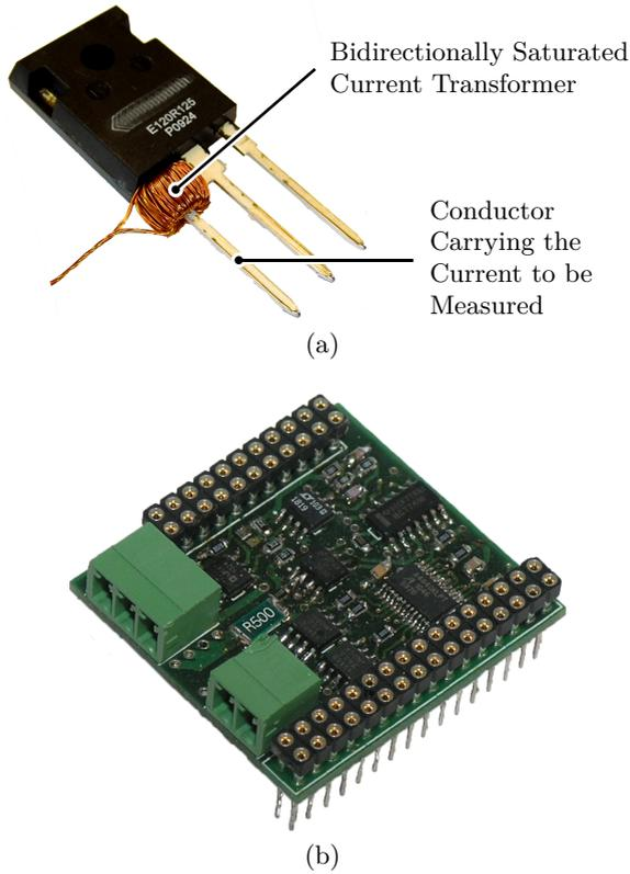
Figure 7.6: (a) Photograph of the bidirectionally saturated current transformer mounted on a discretely packaged SiC power semiconductor switch. (b) Photograph of the PCB with signal and low power electronics to magnetize the current transformer core from its secondary side. The PCB also contains the connectors to the current transformer and to the digital control platform of the overall converter system which employs the system for current measurement.
