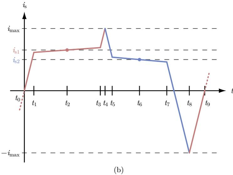
Figure 7.4: Traversing the  $B(H)$  hysteresis loop by proper modulation of the H-bridge connected to the secondary side as shown in Figure 7.3: The different operating points of the bidirectionally saturated current transformer within one pulse period of the H-bridge are shown on the (a) hysteresis loop and (b) secondary current waveform.
