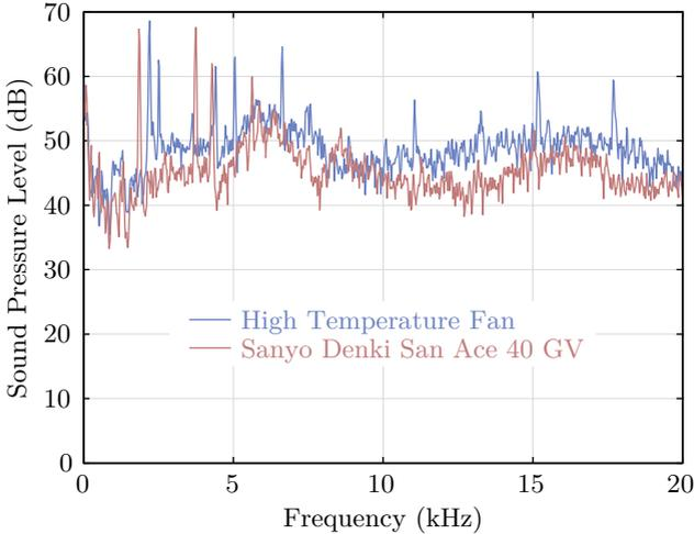
Figure 8.7: Measured sound pressure level over the audible frequency range at 25 °C for the high temperature fan and for the Sanyo Denki San Ace 40 Gv fan. (*cf.* Table 8.2 for calculated total sound pressure level).
