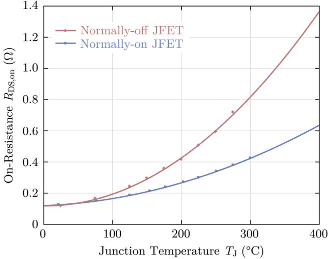
Figure 3.2: Measured and curve fitted temperature dependency of the on-state resistance of the SemiSouth 1200 V normally-off SiC JFET “SJEP120R100” and of the Infineon 1200 V normally-on JFET as a comparison.
