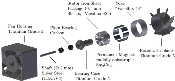
Figure 6.4: Exploded view drawing of high temperature ( $250^{\circ}\text{C}$  /  $500^{\circ}\text{F}$ )  $19'000\text{ min}^{-1}$  BLDC fan for forced air-cooling of advanced automotive power electronics.
