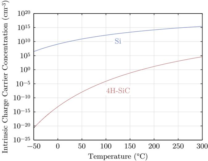
Figure 1.1: Intrinsic charge carrier concentration of silicon and silicon carbide over temperature [17, 18]. The intrinsic charge carrier concentration of SiC is below the respective value of Si up to the melting point of Si at 1420 °C, making significantly higher operating temperatures up to more than 400 °C possible for SiC compared to typically 175 °C for Si (*cf.* Equation (2.1)).
