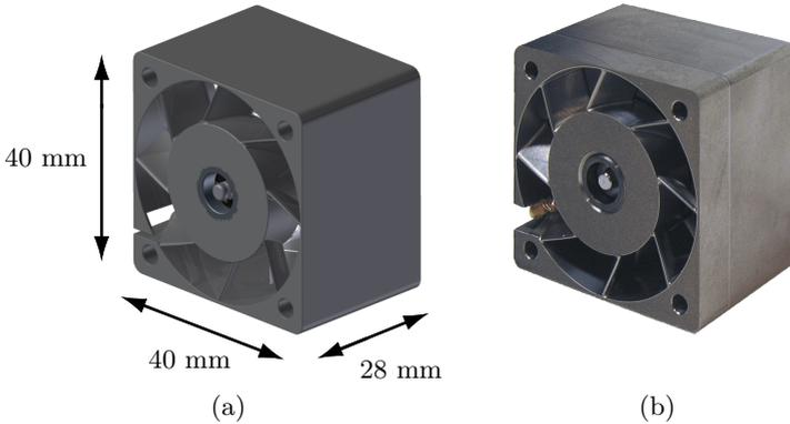
Figure 6.1: (a) CAD picture and (b) photograph of high temperature ( $250\text{ }^{\circ}\text{C} / 500\text{ }^{\circ}\text{F}$ )  $19'000\text{ min}^{-1}$  BLDC fan for forced air-cooling of advanced automotive power electronics.
