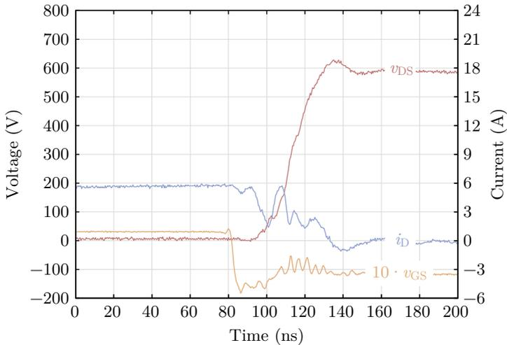
Figure 8.2: JFET switching transients with the proposed gate driver in a test circuit as shown in Figure 8.1. (a) Turn-on and (b) turn-off are finished after 34 ns and 24 ns, respectively. The gate-source voltage waveform shows the negative bias during the off-state and the significantly increased gate voltage during the switching transients.
