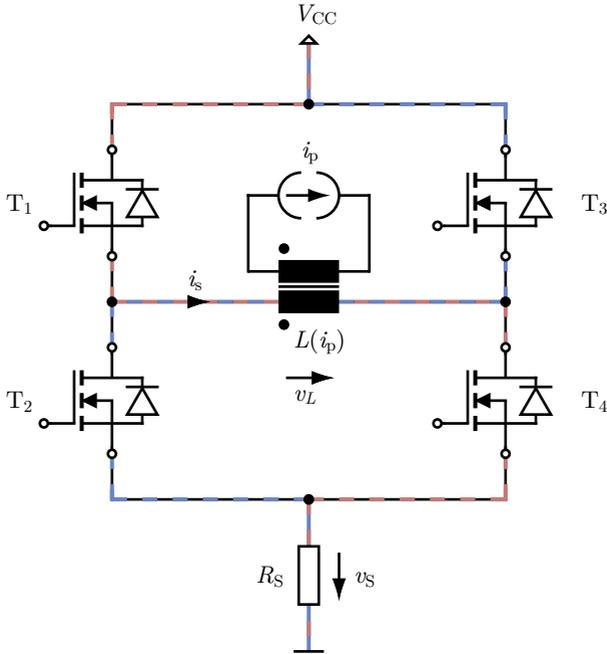
Figure 7.3: Circuit diagram of the current measurement setup: The bidirectionally saturated current transformer is magnetized by a primary current  $i_p$ . The secondary winding on the toroidal core of the transformer is connected to an H-bridge and the secondary current  $i_s$  is measured by a shunt  $R_S$ . The colored current paths correspond to a section of the current waveform shown in Figure 7.4(b).
