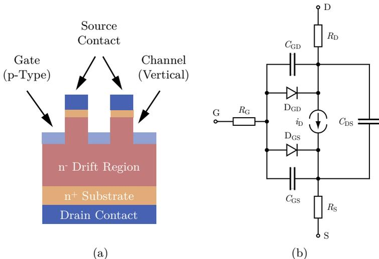
Figure 4.1: 1200 V normally-off SiC JFET: (a) cross-section and (b) equivalent circuit diagram. Notable is with respect to the gate driver design in particular the pn-junction diode at the gate as well as the purely vertical structure of the device leading to an inherently high gate-drain capacitance (*cf.* Section 4.1.1 and Section 4.1.2).
