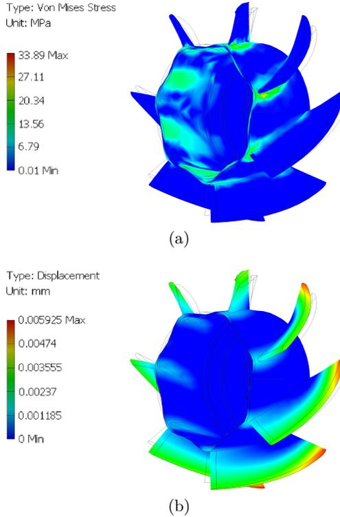
Figure 6.5: FEM simulation of rotor (a) von Mises stress and (b) displacement at a rotational speed of  $19'000 \text{ min}^{-1}$  and an ambient temperature of  $300^\circ\text{C}$ . A safety margin of more than 15 for the maximum stress is included for the designed Titanium Grade 5 rotor.
