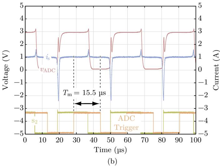
Figure 8.9: Measured waveforms at (a) 25 °C and (b) 250 °C ambient temperature of the magnetic core:  $v_{ADC}$  at the input of the ADC of the DSP, shunt current  $i_s$ , switching signal  $s_2$  and software trigger starting the ADC conversion, with the latter two plotted with a negative offset of 5 V and scaled by a factor of 0.5 for the sake of clarity.
