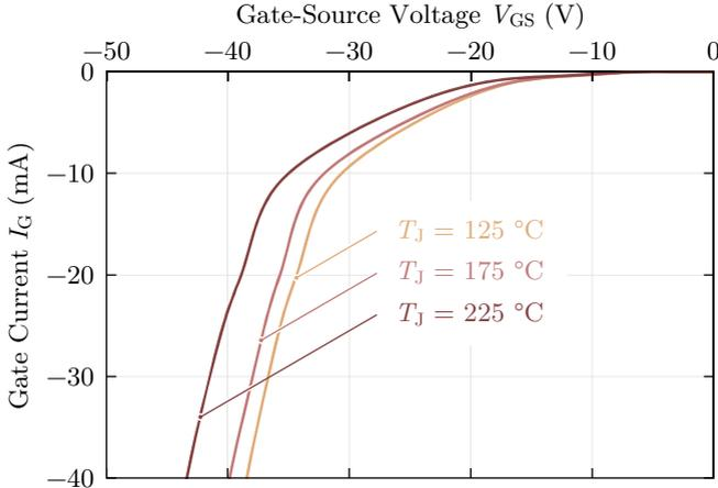
Figure 4.6: Measured reverse gate-source dc characteristic of the 1200 V 40 A normally-off SiC JFET for different junction temperatures  $T_J$ . A bias exceeding -15 V should not be applied to the gate in order to limit the losses during the off-state.
