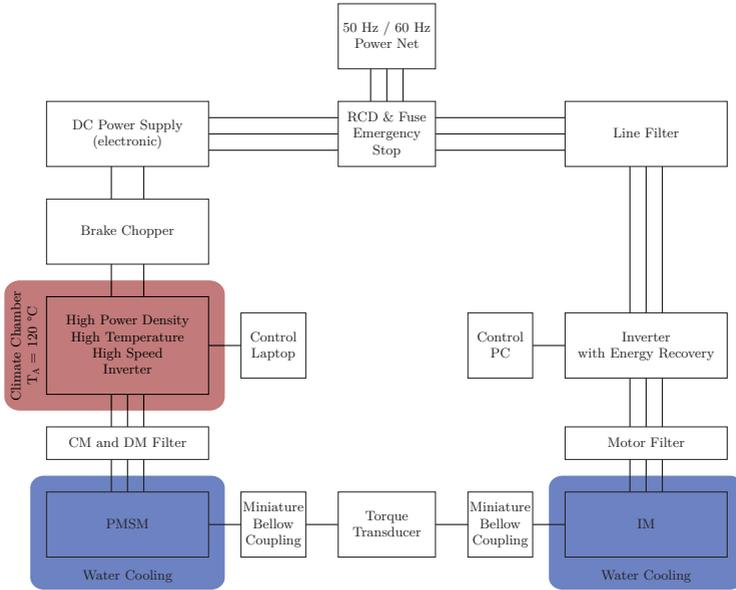
Figure 8.13: Block diagram of the test bench for the high temperature inverter system. The PMSM and IM have a rated power of 10 kW, four poles, and a maximum rotational speed of  $30\,000\text{ min}^{-1}$ .
