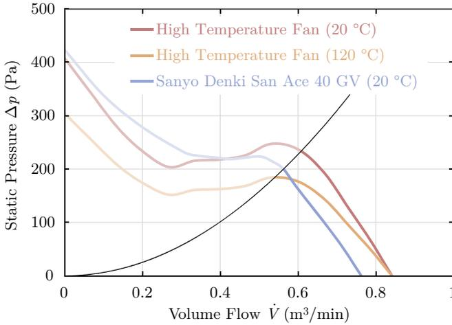
Figure 6.2: Static pressure over volume flow curves for the high temperature fan presented with  $19'000 \text{ min}^{-1}$  at  $20^\circ\text{C}$  and  $120^\circ\text{C}$  as well as for the Sanyo Denki reference fan with  $16'500 \text{ min}^{-1}$ . The fluid dynamic design criteria for the high temperature fan at  $120^\circ\text{C}$  in terms of  $\dot{V}_{\text{max}}$  and  $\Delta p$  is fulfilled for the largest part of the characteristic curve given by the parabola of operation.
