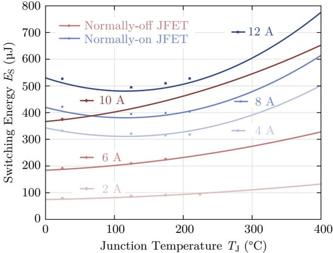
Figure 3.3: Measured and curve fitted switching energies (turn-on and turn-off) for different temperatures and drain currents of the 1200 V normally-off SiC JFETs with an antiparallel SiC diode (Cree “C2D10120”) [69] and an inductive load. The normally-on JFET has got a four times larger die area than the normally-off JFET. The switched voltage is 700 V for both devices.
