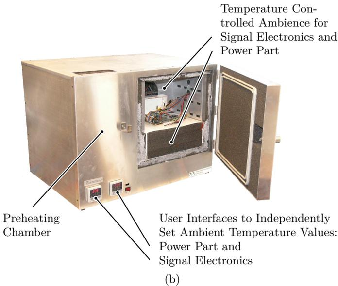
Figure 8.12: (a) 3-phase currents of the inverter driving the PMSM. The currents are almost sinusoidal with very low harmonic distortion due to the high inverter switching frequency of 50 kHz. (b) Photograph of the complete thermal chamber which is used to test the inverter system at 120 °C ambient temperature.
