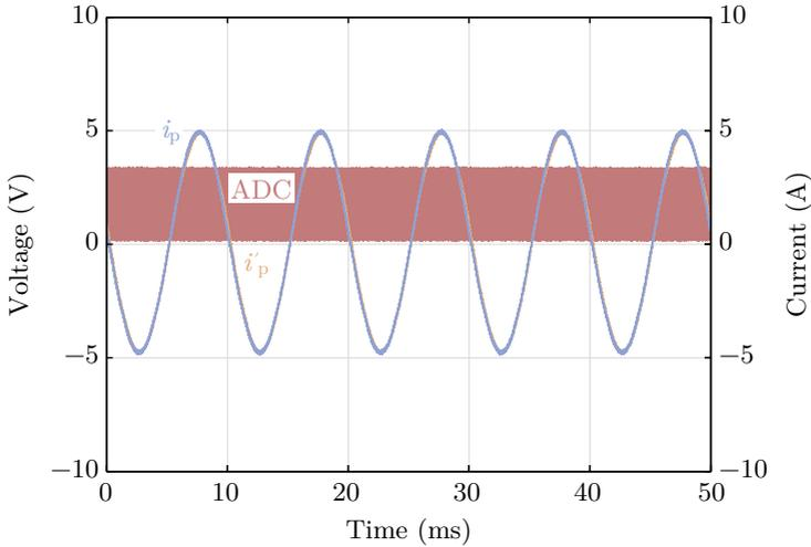
Figure 8.8: The primary current measured with a wide band power analyzer (waveform denoted with  $i_p$ ) and with the presented bidirectionally saturated current transformer (waveform denoted with  $i'_p$ ). Also shown is the signal triggering the ADC.
