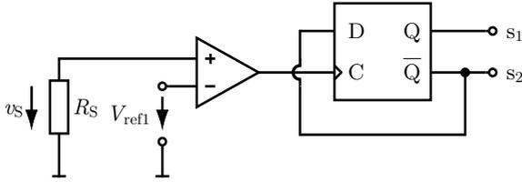
Figure 7.9: Generation of the switching signals for the H-bridge by comparing the shunt voltage  $v_S$  with a reference voltage  $V_{\text{ref1}}$ : The output of the comparator (National Semiconductor “LM360”) is fed to the clock input of a D flip-flop (Texas Instruments “CD74HCT74M”), the inverted output of which is connected to the D input of the flip-flop.
