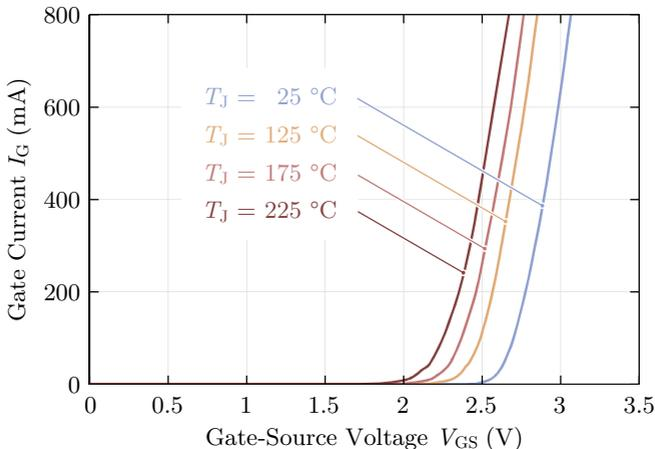
Figure 4.2: Measured gate-source dc characteristic of the 1200 V 40 A normally-off SiC JFET for different junction temperatures  $T_J$ . During the on-state of the normally-off SiC JFET, the gate-source voltage  $V_{GS}$  should not exceed 3 V in order to avoid large currents flowing into the gate.
