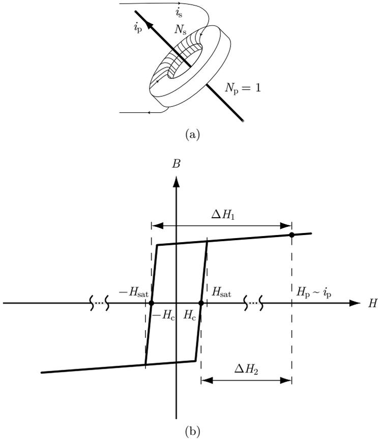
Figure 7.2: (a) Basic physical setup of the bidirectionally saturated current transformer: The (primary) current  $i_p$  to be measured is fed through a toroidal core that also carries a secondary winding. (b) Basic measurement principle: The primary current is determined using the mean value of the secondary currents that are needed to reach the coercive magnetic field strengths  $\pm H_c$  of the hysteresis loop.
