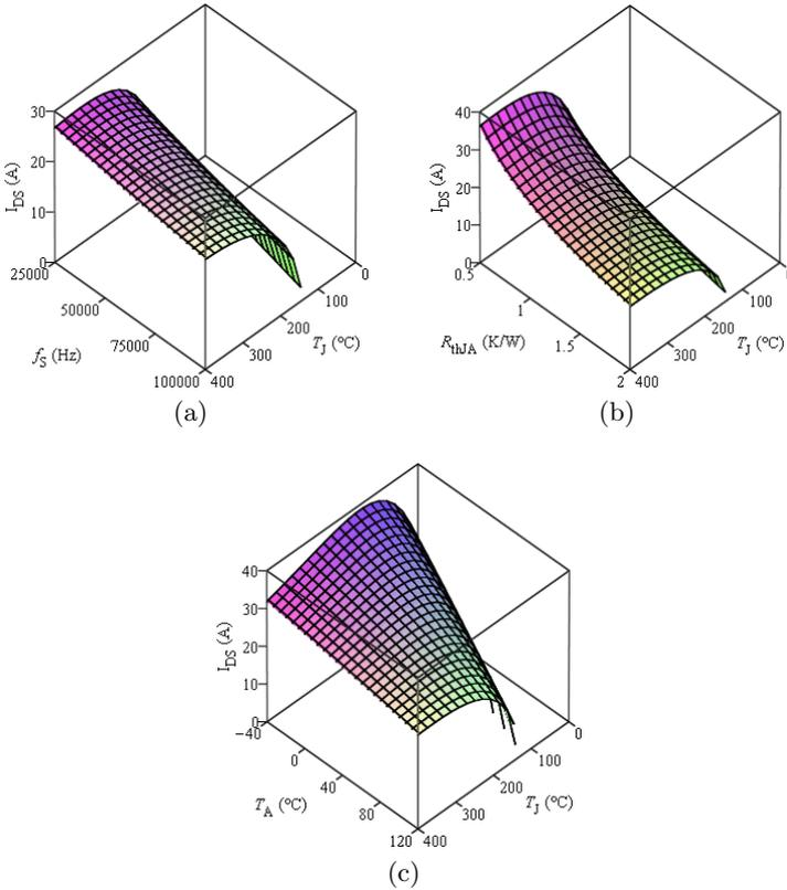
Figure 3.6: Admissible drain current as a function of the junction temperature as well as (a) ambient temperature, (b) switching frequency, and (c) thermal resistance for four 1200 V normally-off SiC JFET connected in parallel.
