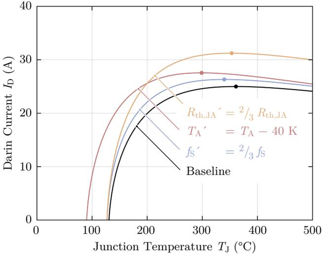
Figure 3.7: Drain current as a function of junction temperature with variations in the ambient temperature  $T_A$ , the switching frequency  $f_s$ , and the thermal resistance  $R_{th,JA}$  for four paralleled dies of the 1200 V normally-off SiC JFET. The respective values for the maximum drain current and corresponding junction temperature is indicated by a dot.
