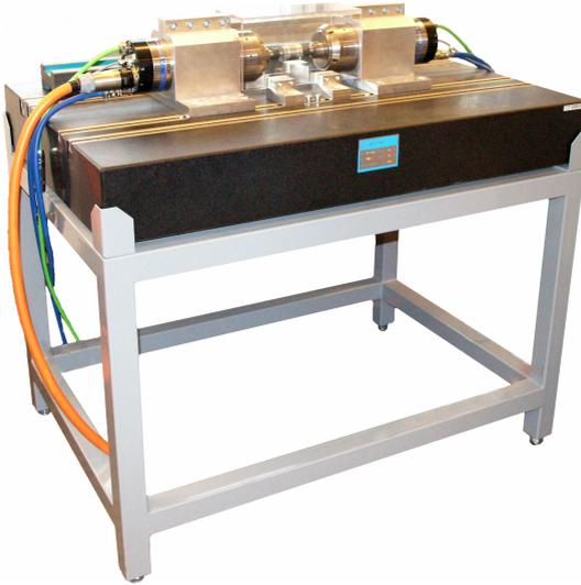
Figure 8.14: Photograph of the test bench equipped with a PMSM and an IM, a miniature bellow coupling, a transparent safety hood covering all rotating parts, a marble ruler as an adjustment fixture, and a marble machine base.
