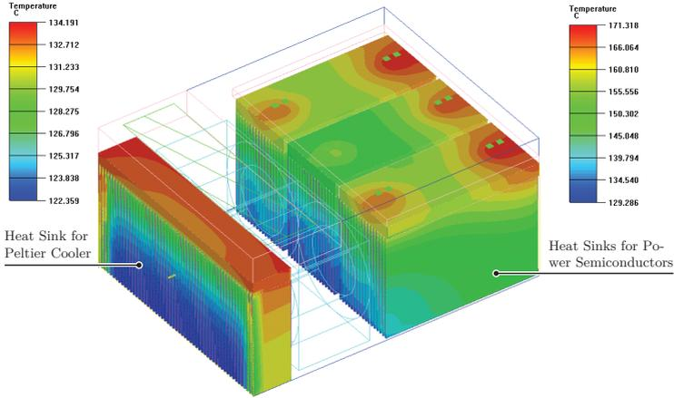
Figure 5.4: Thermal simulations of the cooling of the power semiconductors and the Peltier cooler. The ambient temperature is 120 °C, the junction temperature of the power semiconductors is set to 250 °C (relevant operating point for the design of the electronics cooling) and the power dissipated by the Peltier device is 50 W.
