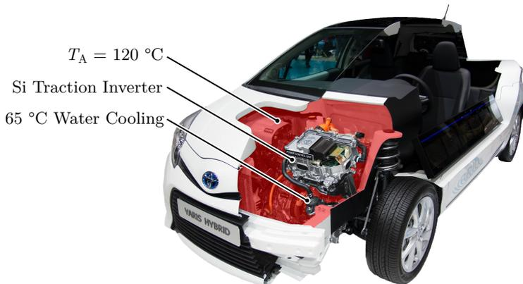
Figure 1.2: Toyota Hybrid Synergy Drive in a Yaris Hybrid of the model year 2012: Industrial example of a traction inverter with Si IGBTs which is placed under the engine hood with ambient temperatures up to  $120\text{ °C}$  and hence requires a low temperature water cooling circuit. (Photograph taken at the world premiere of the Toyota Yaris Hybrid at the 82nd Geneva International Motor Show in March 2012.)
