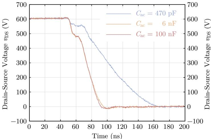
Figure 8.3: Drain-source voltage of  $T_{LS}$  during turn-on for different values of  $C_{ac}$  (cf. Figure 4.7). As expected, a smaller value than  $C_{ac} = 6$  nF leads to a significantly slower turn-on while an increase does not yield a significant gain in switching speed.
