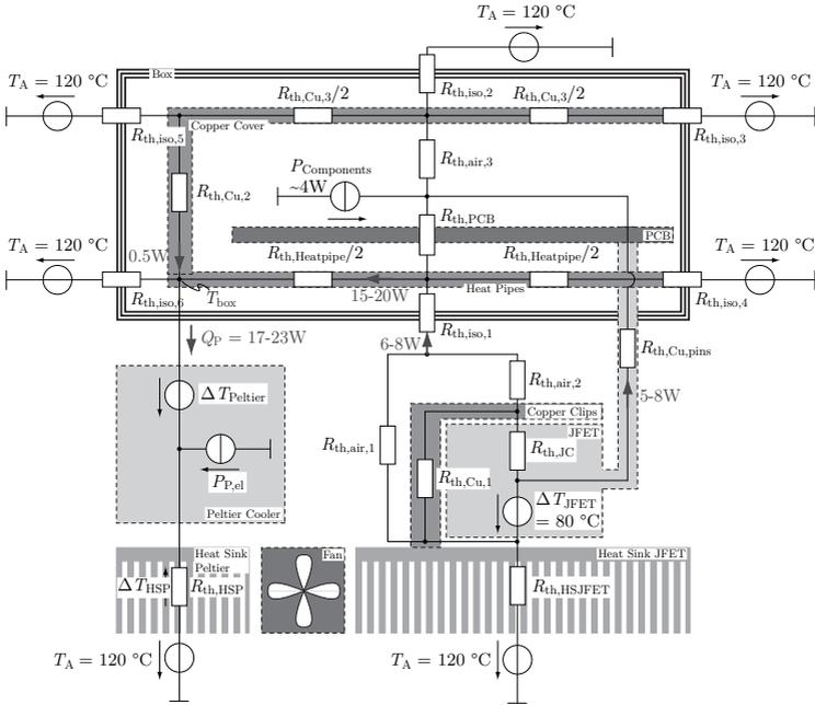
Figure 5.6: Equivalent circuit model to calculate the heat induced into the control electronics box (20 W) and to derive a model for the Peltier cooling.
