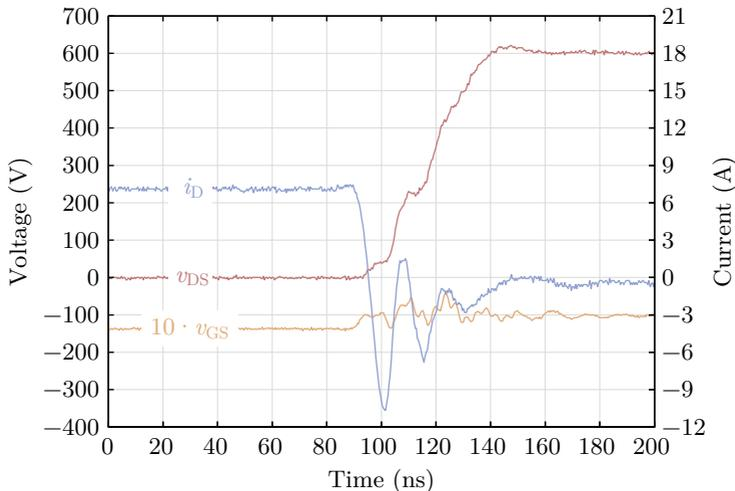
Figure 8.4: Robustness against the Miller effect: It can be seen, that the gate-source voltage is less than  $-5\text{ V}$ , so that a safety margin of more than  $5\text{ V}$  to an accidental turn-on of the JFET is maintained in the whole switching interval.
