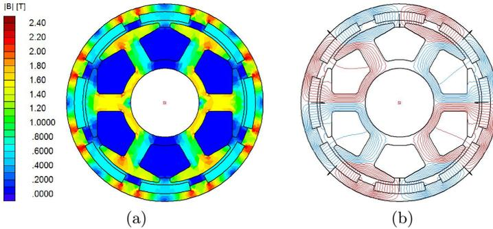
Figure 6.3: (a) Flux density distribution under full load condition. The flux density in the stator and yoke is less than 2.1 T which is below the saturation limit of 2.35 T of the employed iron cobalt material (*cf.* Section 6.3.2 and Section 6.3.4). (b) Magnetic field lines under no load condition of the BLDC machine.
