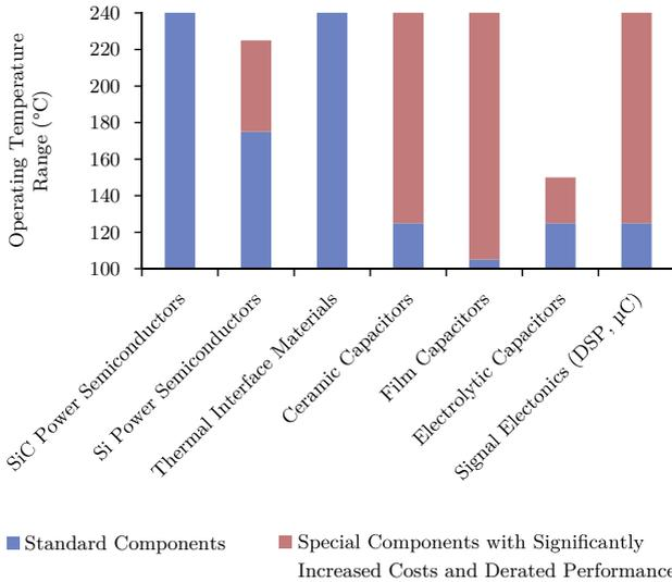
Figure 5.1: Overview over operating temperature ranges of the main components of the investigated inverter system. The significantly derated performance of special components refers to the much higher on-resistance of silicon-on-insulator-type Si power semiconductors, the much lower energy density of high temperature capacitors or the limited signal processing capability of high temperature DSPs.
