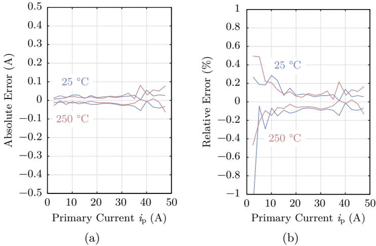
Figure 8.10: Minimum and maximum (a) absolute and (b) relative measurement error of the proposed current measurement system over the full measurement range after initial calibration of the setup to compensate for the linearity error introduced by tolerances of resistance values.
