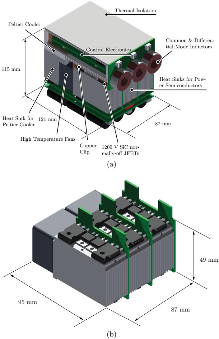
Figure 5.7: (a) CAD representation of the investigated inverter system. The overall volume including dc-link capacitors and active control electronics cooling is 1.21 leading to an overall power density of  $8.3 \text{ kW/l}$ . (b) CAD representation of the power part of the inverter system with a volume of 0.41 (including the fans).
