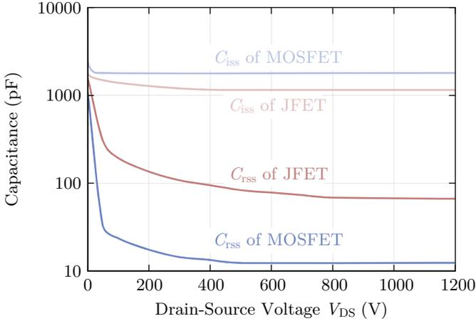
Figure 4.5: Comparison of the measured input and reverse transfer capacitance ( $C_{iss}$  and  $C_{rss}$ , respectively) of a 1200 V 40 A normally-off SiC JFET and a typical SiC MOSFET (type: Cree, Inc. “CMF20120D” [90]) with similar voltage and current rating showing the high gate-drain and low gate-source capacitance of the JFET.
