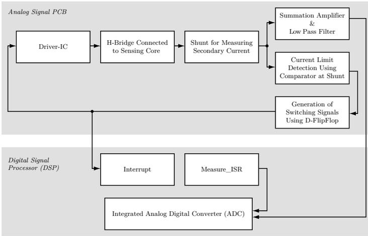
Figure 7.8: Signal flow diagram for the analog control of the current measurement system and for the measurement routine within a DSP.
