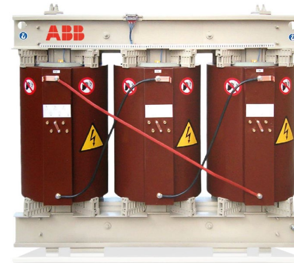
1 MVA – 12 kV / 400 V @ 2600 kg 0.2%/1% Losses @ No/Rated Load
