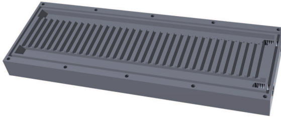
Fig. 5.41: Possible Design of a water cooler using a horizontal fin structure.
