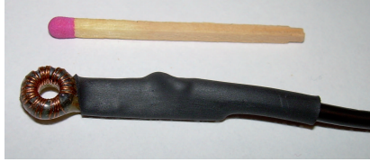
Fig. 5.6: Constructed AC current transformer with a sensitivity of 100 mV/A to measure the drain source current I_{DS} of the MOSFET.
