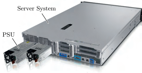
Fig. 1.3: Lenovo ThinkSystem® server solution from the rear-side perspective, with highlight to the two available power supply units (PSUs) for a 1+1 redundancy scheme.
