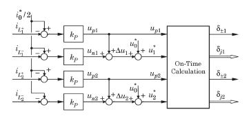
Fig. 8. Control structure for the dc-link current balancing of two parallelconnected rectifier systems based on the dc/dc equivalent circuit given in Fig. 5.
