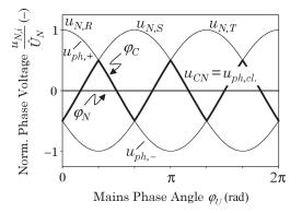
Fig. 6. Normalized mains phase voltages  $u_{N,R}$ ,  $u_{N,S}$ , and  $u_{N,T}$ ; clamped voltage  $u_{\text{ph,cl.}}$  at the right-hand terminals of the dc-link inductors during the free-wheeling state; voltages  $u_{\text{ph},+}$  and  $u_{\text{ph},-}$ ; and voltage between common point C and mains neutral point N.
