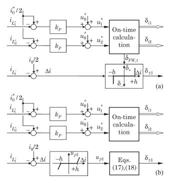
Fig. 10. Modified control structures for balancing the dc-link inductor currents based on a bang-bang control.  $\pm h$  represents the width of the hysteresis. (a) Control structure 1: fixed duration of the additional free-wheeling state. (b) Control structure 2: variable on-time of the additional free-wheeling state.
