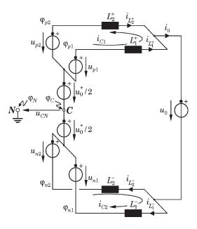
Fig. 5. DC/DC equivalent circuit of two parallel-connected buck-type rectifier systems showing the circulating currents  $i_{C1}$  and  $i_{C2}$  that represent the dc-link current unbalance and the potentials  $\varphi_{pm}$  and  $\varphi_{nm}$ , m = 1, 2, on the left-hand side of the dc-link inductors  $L_{12}^{\pm}$ . The voltage sources  $u_0^*/2$  are representing the buck-stage output voltages being necessary for generating the system output voltage  $u_0$ .
