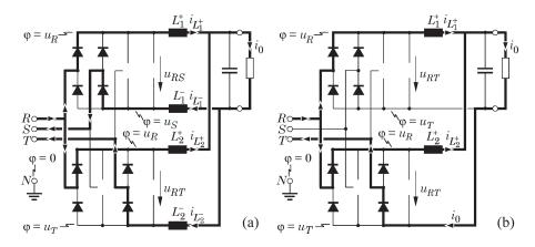
Fig. 3. Necessity for splitting of dc-link inductors to positive and negative dc-link rails for parallel-connected rectifier systems. (a) Splitted dc-link inductors to positive and negative dc-link rails. (b) DC-link inductors placed only in the positive dc-link rails resulting in overloading system 2 and in a different input current formation.
