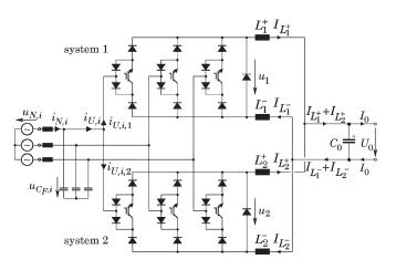
Fig. 1. Power circuit of the parallel connection of two three-phase/switch buck-type unity-power-factor PWM rectifier systems.
