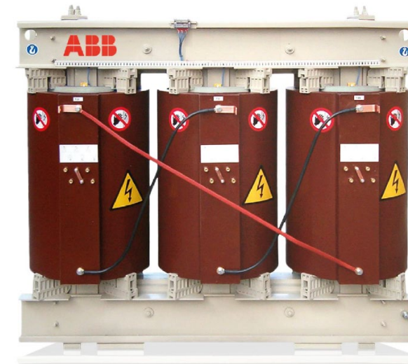
1 MVA – 12 kV / 400 V @ 2600 kg 0.2%/1% Losses @ No/Rated Load
