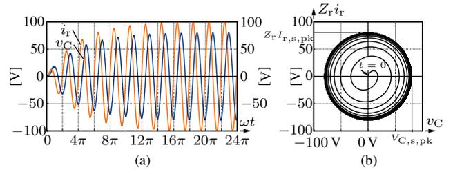
Fig. 3. (a) Response of the resonant tank of Fig. 1 to a sinusoidal excitation; (b) corresponding phase diagram.
