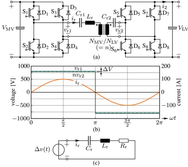
Fig. 1. (a) HC-DCM-SRC topology; (b) simulated current and voltage waveforms for  $L_r = 16 \mu\text{H}$ ,  $C_r = 25 \mu\text{F}$ ,  $R_r = 130 \text{ m}\Omega$ ,  $V_{\text{MV}} = 800 \text{ V}$  and  $P_{\text{out}} = 50 \text{ kW}$ ; (c) simplified and primary side referred converter model [13].
