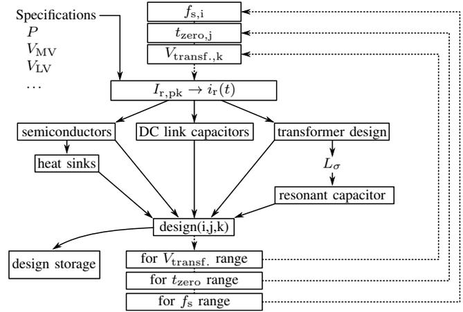
Fig. 15. Visualization of the procedure that calculates the design points used to find the Pareto front shown in Fig. 16.
