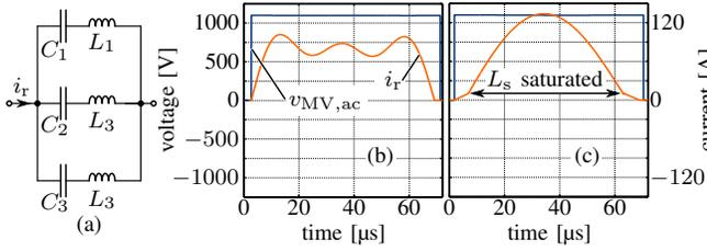
Fig. 13. (a) Extended resonant tank where branch 1 is tuned to  $f_0 = 7500$  kHz, branch 2 to  $3f_0$  and branch 3 to  $5f_0$  and (b) resulting current waveform. (c) shows the current shape when a saturable inductor is connected in series to the normal LC resonant tank instead.
