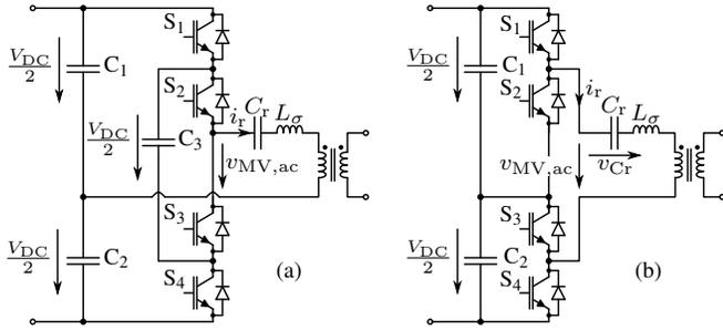
Fig. 6. Other realization options for the MV side bridge that allow for using 1.7 kV IGBTs for  $V_{DC} = 2.2$  kV; (a) adds a flying capacitor while (b) uses a DC offset of  $V_{DC}/2$  on the resonant capacitor [20].
