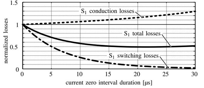
Fig. 10. Influence of the zero current interval duration on the semiconductor losses for  $f_s = 7.5\ \text{kHz}$  and  $T_j = 125^\circ\text{C}$ . Note that the optimum is shifted to the left and upwards if other losses related to rms current are included.
