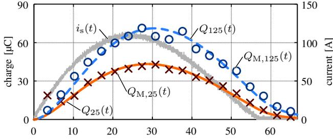
Fig. 9. Behavior of the stored charge for the FF150R17KE4 IGBT at  $T_j = 25^\circ\text{C}$  and  $T_j = 125^\circ\text{C}$ .  $Q_{M,25}(t)$ ,  $Q_{M,125}(t)$  are measurements and  $Q_{25}(t)$ ,  $Q_{125}(t)$  are obtained with (14) and  $k_s$ ,  $\tau$  as given in Table II.
