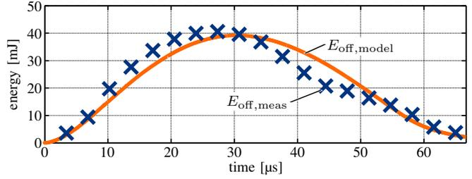
Fig. 14. Measurement and estimate of the turn-off losses in  $S_1$  at  $T_j = 125^\circ\text{C}$ . The  $\Delta t$  values used for the measurements are the same as in Fig. 9.
