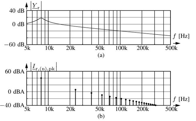
Fig. 2. (a) Admittance of the resonant tank ( $L_r = 16 \mu\text{H}$ ,  $C_r = 25 \mu\text{F}$ ,  $R_r = 130 \text{ m}\Omega$ ); (b) calculated spectrum of  $i_r$ :  $I_{r,(1),\text{pk}}$  is 34 dB higher than  $I_{r,(3),\text{pk}}$ . The spectrum of Fig. 2(b) corresponds to the current depicted in Fig. 1(b), which is almost sinusoidal.
