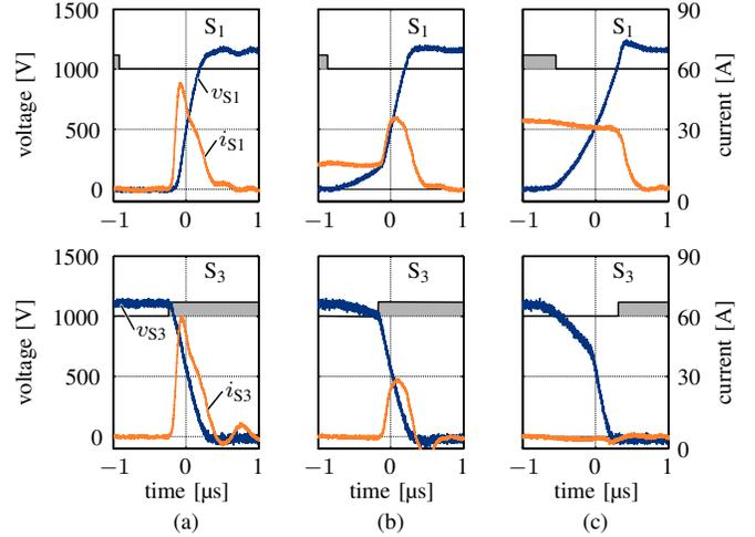
Fig. 11. The commutation process changes with increasing magnetizing current from (a) pure ZCS via (b) a mixed form to (c) soft-switching. The measurements were taken with a zero current interval of about  $2\ \mu\text{s}$  and an effective interlock time of about  $0.8\ \mu\text{s}$ ; the gate signals are indicated qualitatively.
