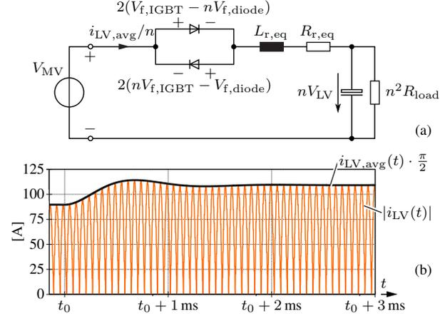
Fig. 5. (a) Small signal model of the HC-DCM-SRC; (b) simulated response to a load step (45 kW  $\rightarrow$  55 kW) at  $t_0$ : the peak values of the oscillating current, obtained from a simulation of the circuit shown in Fig. 1, are in good agreement with the envelope (thick line), which is obtained by scaling the average current,  $i_{LV,avg}$ , of Fig. 5(b) with a factor of  $2/\pi$ . Component values:  $L_{r,eq} = 39.5 \mu\text{H}$ ,  $R_{r,eq} = 160 \text{ m}\Omega$ .
