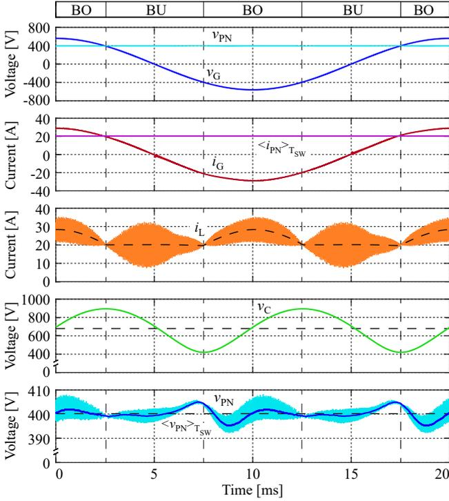
**Fig. 5:** Simulated steady state waveforms for the proposed buck+boost PFC rectifier with iSPPB showing the grid and DC-link waveforms as well as the operating mode, the inductor current  $i_L$ , the buffer capacitor voltage  $v_C$  and the DC-link voltage  $v_{PN}$  together with its local average  $\langle v_{PN} \rangle_{T_{SW}}$  within one grid period  $T_G = 20$  ms. The corresponding references are indicated by dashed lines.
