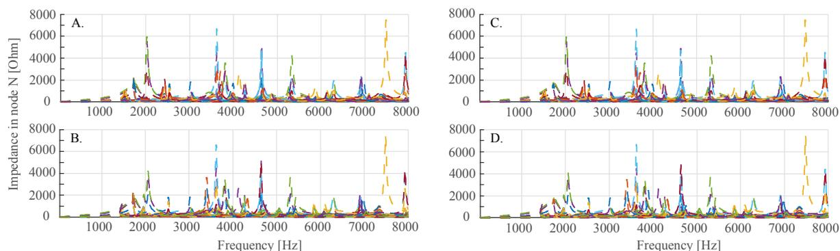
Fig. 6: Frequency scan, results for a phase: current network, current network with opened switch in node 36, the network with a HVDC link, the network with a HVDC link and with opened switch in node 36.
