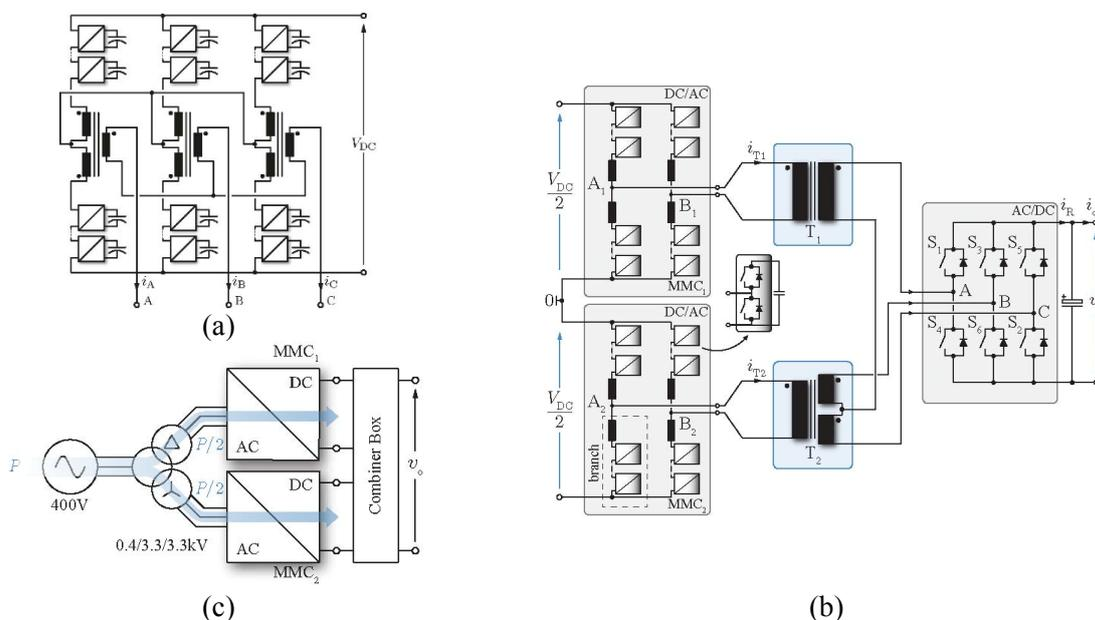
Fig. 1: (a) GIMC, featuring integrated magnetic structure into the MMC structure. (b) High-power DC-DC converter utilizing Scott transformer connection. (c) MMC-based MVDC amplifier.
