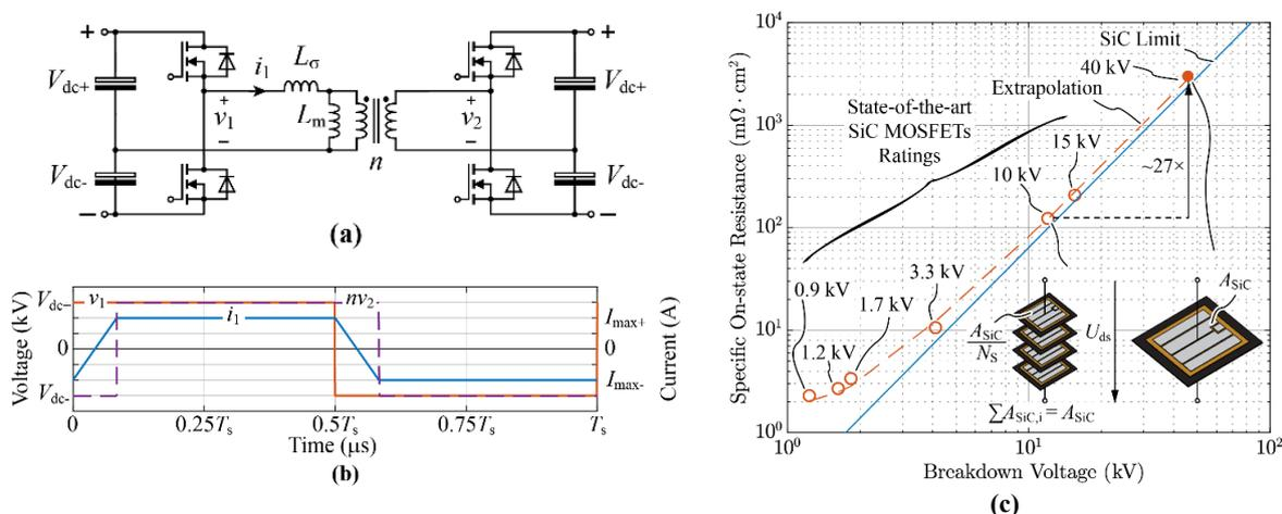
Fig 2: (a) DAB-type DC–DC converter employing a MV SiC half-bridge at the input side. (b) Simulated transformer primary and secondary side quantities (magnetizing current neglected). (c) Specific on-state resistance of SiC MOSFETs and SiC theoretical limit based on [7]. Bottom-right: starting point for the comparison of the specific on-state resistances of a considered 40 kV SiC MOSFET and four 10 kV SiC MOSFETs ( $N_s = 4$ ,  $U_{ds} = 40$  kV).
