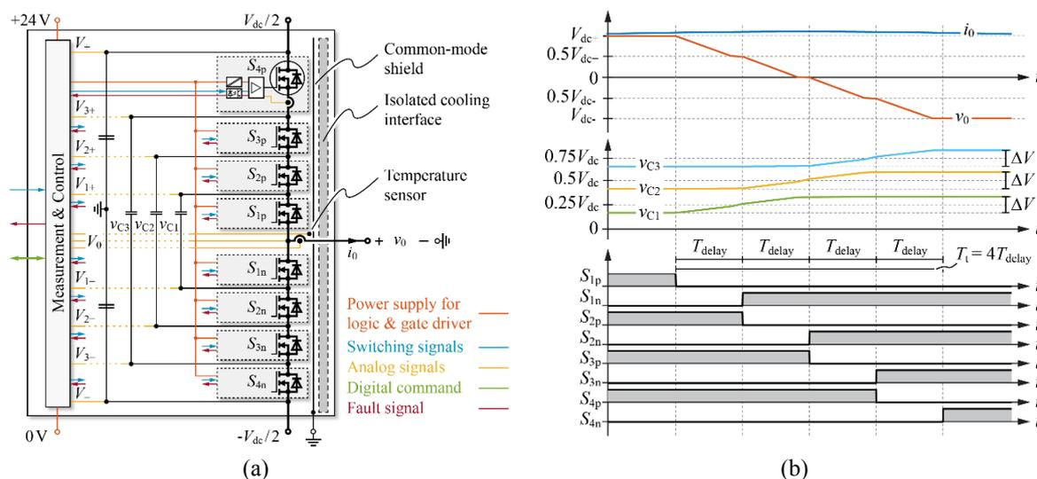
Fig. 3 (a) Proposed Flying Capacitor Q2L SiC Super-Switch Intelligent Power Module (SiC-SS-IPM) with 10kV SiC power MOSFETs [13]. (b) Simulation results for Q2L operation of a 5L-FCC bridge leg: time intervals and simulated waveforms of output current  $i_0$  and output voltage  $v_0$ , flying capacitor voltages  $v_{C1}$ - $v_{C3}$ , and gate signals.
