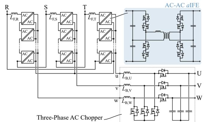
**Fig. 15.** Three-phase IFE SST for AC-AC applications.
