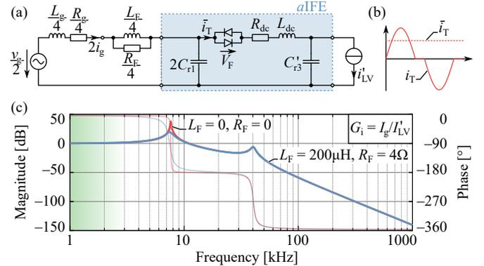
**Fig. 6.** (a, b) Dynamic equivalent circuit of the  $aIFE$  (HC-DCM SRC) including filter and grid impedances, and (c) corresponding transfer function from the boost stage inductor current to the grid current,  $G_i(s)$ , using the data from **Tbl. IV** and  $L_\sigma = 10 \mu\text{H}$ .
