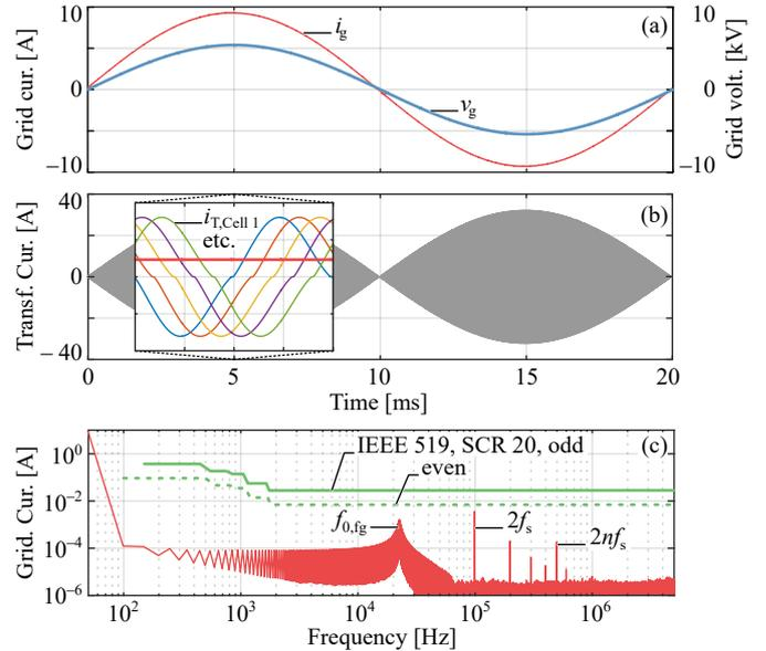
**Fig. 8.** Simulation results of a single-phase ISOP system (cf. **Fig. 7a**), where the boost stage is modeled as a current source, and with  $L_g = 690 \mu\text{H}$ ,  $R_g = 22 \text{ m}\Omega$ ,  $L_F = 200 \mu\text{H}$ , and  $R_F = 10 \Omega$ .
