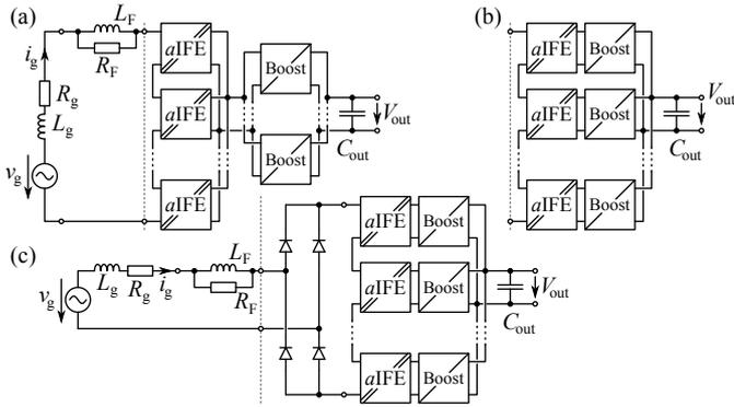
**Fig. 7.** Three ISOP configuration variants of the IFE topology; (a) common [AC] bus and single boost stage employing interleaved sub-units, (b) one boost stage per *aIFE* cell, and (c) common input rectifier using high-voltage semiconductors (possibly realized as an active rectifier by adding anti-parallel switches to the diodes).
