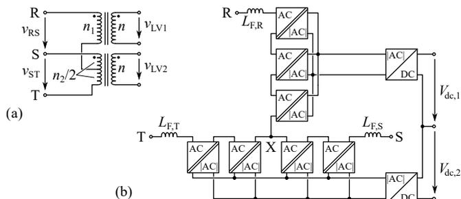
Fig. 16. (a) Magnetic Scott transformer, (b) IFE-based Scott transformer configuration.
