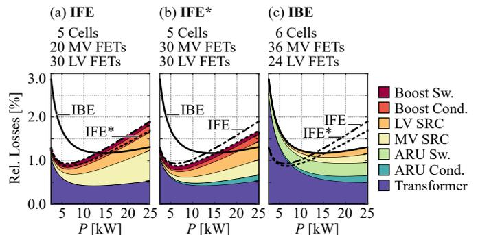
**Fig. 13.** Relative semiconductor and transformer losses for the three systems considered in the case study.
