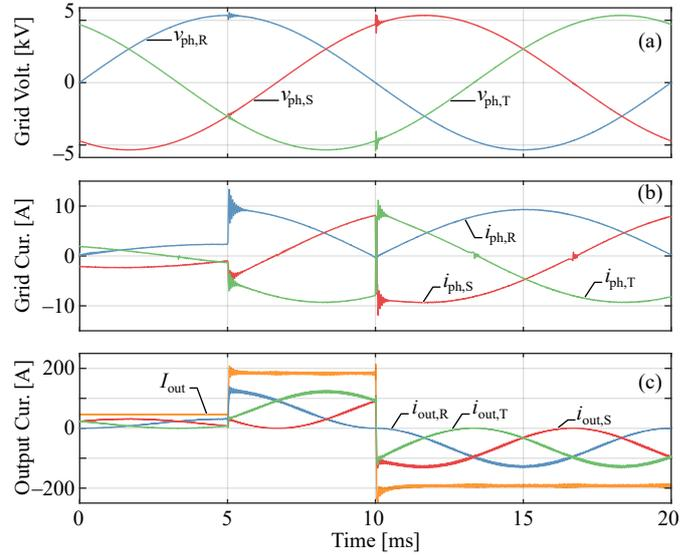
**Fig. 14.** Simulation of a three-phase IFE SST system including transients.
