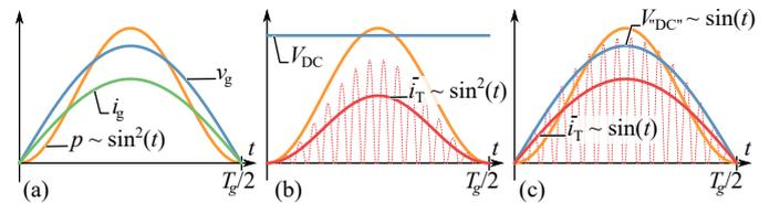
**Fig. 11.** Power transfer in (a) a single-phase grid, (b) in an IBE, and (c) an IFE system.
