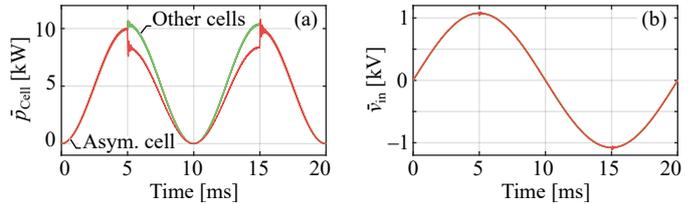
**Fig. 9.** Simulated self-balancing of the cells in ISOP configuration; (a) shows the power distribution between the cells, and (b) shows the sharing of the input voltage. Note that the waveforms show local average values.
