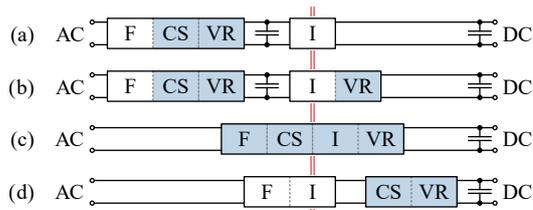
**Fig. 1.** Partitioning of the tasks required to perform isolated PFC: folding (F), current shaping (CS), isolation (I), and output voltage regulation (VR). A shaded background indicates a controllable stage.
