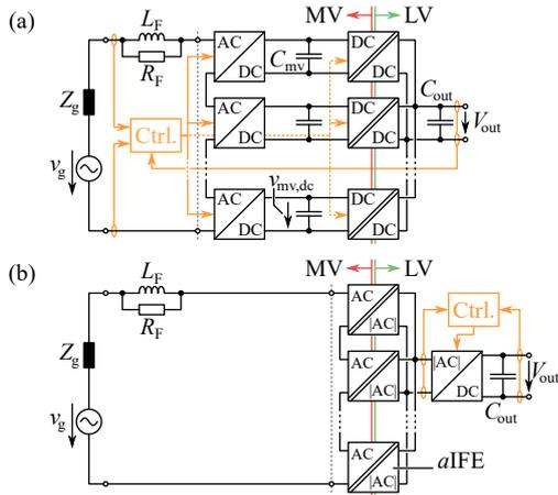
Fig. 2. (a) IBE and (b) IFE systems in ISOP configuration.
