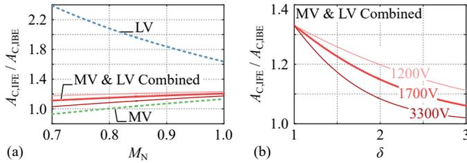
**Fig. 12.** Ratio of the chip area requirements of IFE and IBE systems as a function of the nominal modulation index,  $M_N$  in (a), and in (b) as a function of  $\delta$  in  $r_{on} \propto V_B^\delta$  for  $M_N = 0.8$ . For the combined metric,  $u = 0.66$ ,  $f_s = f_0$ ,  $V_{LV} = 400$  V is assumed, and three different MV semiconductor blocking voltages are considered.
