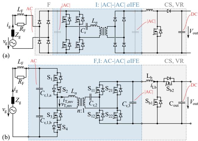
**Fig. 4.** (a) Unidirectional and (b) bidirectional single-cell IFE power circuit topologies. Note that  $C_{r,1,a}$ ,  $C_{r,1,b}$ ,  $C_{r,2}$ , and  $C_{r,3}$  are resonant capacitors, not DC link capacitors.
