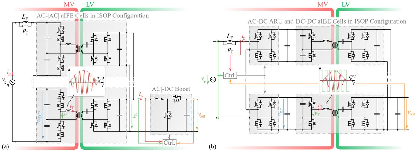
**Fig. 10.** Power circuits of the IFE (a) and the IBE (b) MVAC-LVDC SSTs considered in the comparative evaluation. Note that the number of cascaded cells is different for the two systems in practice (cf. (2)), and that the boost stage of the IFE system would be realized from several smaller boost stages using interleaving.
