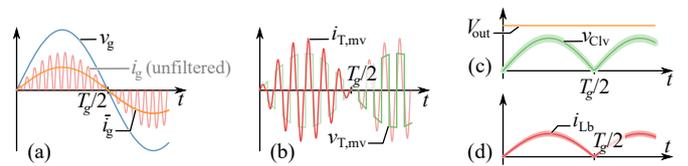
**Fig. 5.** Key waveforms (simplified) of the IFE topology shown in **Fig. 4b**, where a very low switching frequency is assumed for illustration purposes.
