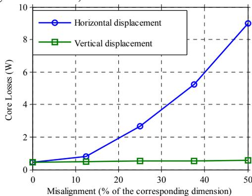
Fig. 14. Increase of the core losses when the core halves are displaced.
