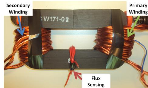
Fig. 15. Transformer built for testing extra losses due to orthogonal flux.
