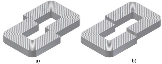
Fig. 12. Displacement of the core halves. a) Horizontal direction, b) vertical direction.
