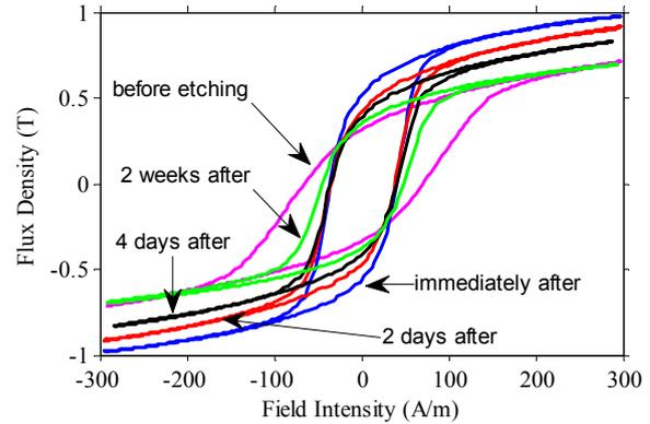
Fig. 5. BH curves of the HB1 core measured at different times.
