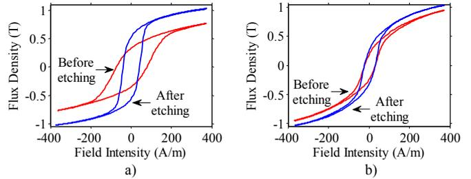
Fig. 4. BH curve of amorphous cores before and after etching, at 1.25kHz. a) HB1 material. b) SA1 material.
