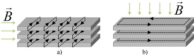
Fig. 10. Eddy currents in tape wound cores. a) Parallel flux density. b) Orthogonal flux density.
