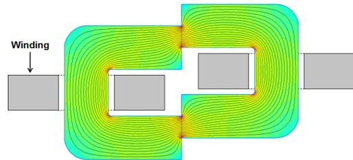
Fig. 13. Flux behavior for horizontal displacement of the cores halves. Colors represent the flux density inside the core.
