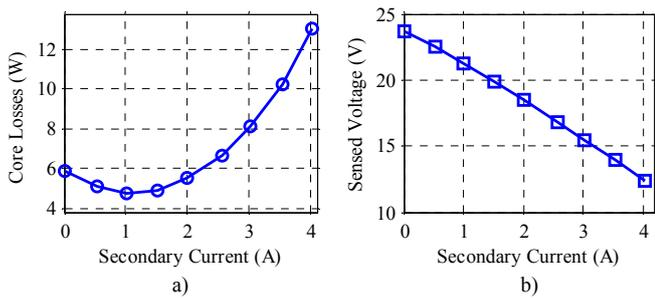
Fig. 16. a) Core loss increase in the tested transformer. b) Sensed voltage related to the flux flowing close to the middle of the bottom leg (Fig. 15).
