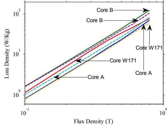
Fig. 11. Core losses in nanocrystalline cut cores, with and without air gap. Dashed lines: With air gap. Solid Lines: No air gap.
