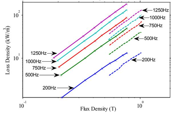
Fig. 3. Core losses of HB1 amorphous core before etching (solid lines) and after etching (dashed lines), at different frequencies.
