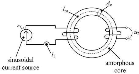
Fig. 2. Basic test setup.
