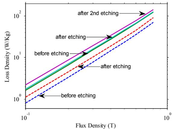
Fig. 9. Measured loss density of different nanocrystalline cores, before and after etching, for triangular flux at 20kHz. Dashed lines: Core A. Solid Lines: Core B.
