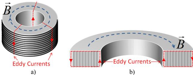
Fig. 7. Eddy currents in the presence of short circuits in the a) cylindrical core; b) toroidal cut core.
