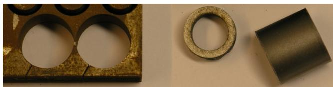
Fig. 1. Picture of a laminated block of HB1 amorphous iron and the cylindrical cores cut out using EDM.
