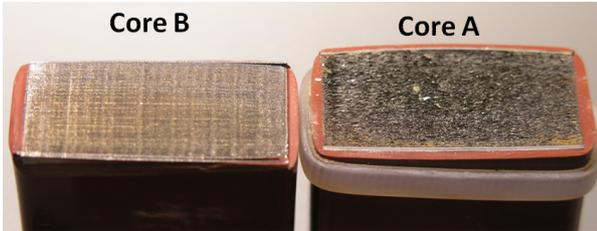
Fig. 6. Toroidal nanocrystalline core cut using EDM (left) and using a thin metal saw (right).
