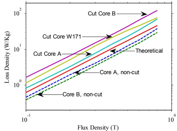
Fig. 8. Measured loss density of different nanocrystalline cores, before and after cutting, for triangular flux at 20kHz.
