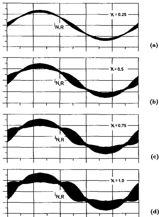
**Fig. 6:** Time behavior of an inverter output phase current for different values of the parameter  $\kappa$  which characterizes the relative amplitude (related to the amplitude  $\hat{I}_N$  of the output current fundamental) of the output current ripple;  $\kappa = 0.25, 0.5, 0.75$  and  $1.0$  (cf. (a) - (d)); simulation parameters:  $\cos \varphi = 1, M = 1.0$
