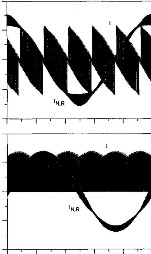
**Fig.4:** Time behavior of the inverter input current  $i$  and the output phase current  $i_{N,R}$  within a fundamental period of the converter output voltage for  $\cos \varphi = 0$  (cf. (a)) and  $\cos \varphi = 1$  (cf. (b)).
