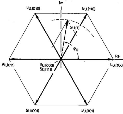
Fig.2: Space vectors of the inverter output voltage assigned to the active inverter switching states and to the non-voltage-forming switching states (000) and (111); furthermore shown: inverter output voltage reference value  $\underline{u}_{U,(1)}$  which has to be formed in the average over a pulse half period of position  $\varphi_U$ ;  $\underline{u}_{U,(1)}$  is associated with the fundamentals of the pulse-width modulated inverter output phase voltages  $u_{U,i}$ ,  $i = R, S, T$ .
