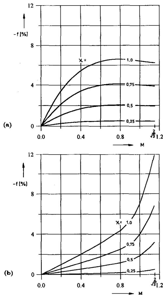
**Fig. 7:** Relative error  $f$  of the analytical calculation of the capacitor current stress  $I_{C,rms,1}$  as caused by the PWM inverter (cf. Eq.(28)) from the results of a digital simulation in dependency on the modulation index  $M$  and the relative amplitude  $\kappa$  of the inverter output current ripple for  $\cos \varphi = 1$  (cf. (a)) and  $\cos \varphi = 0$  (cf. (b)).
