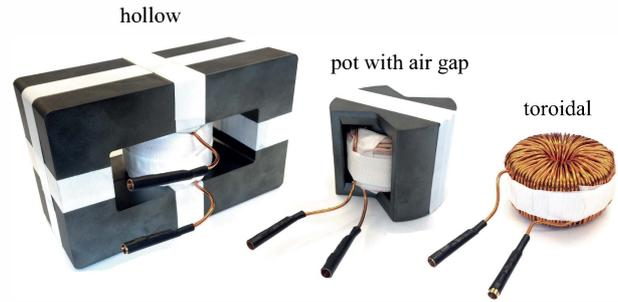
Figure 4. Picture of the inductors used to verify the winding loss model. Instead of a cylindrical hollow core, four C-shaped ferrite cores are used to resemble the same magnetic field distribution in the winding as it would occur in a real cylindrical core.
